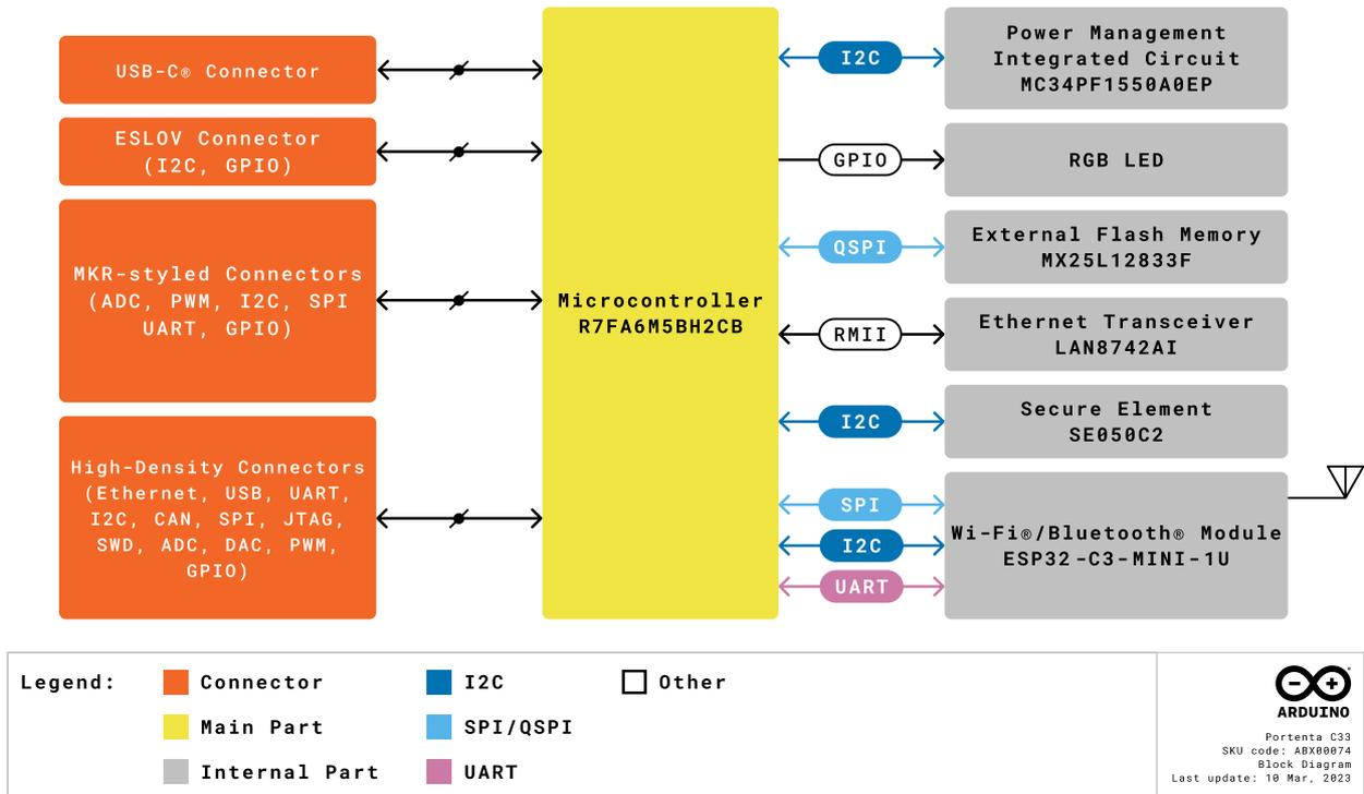
Figure 3. High-level architecture of the Portenta C33
