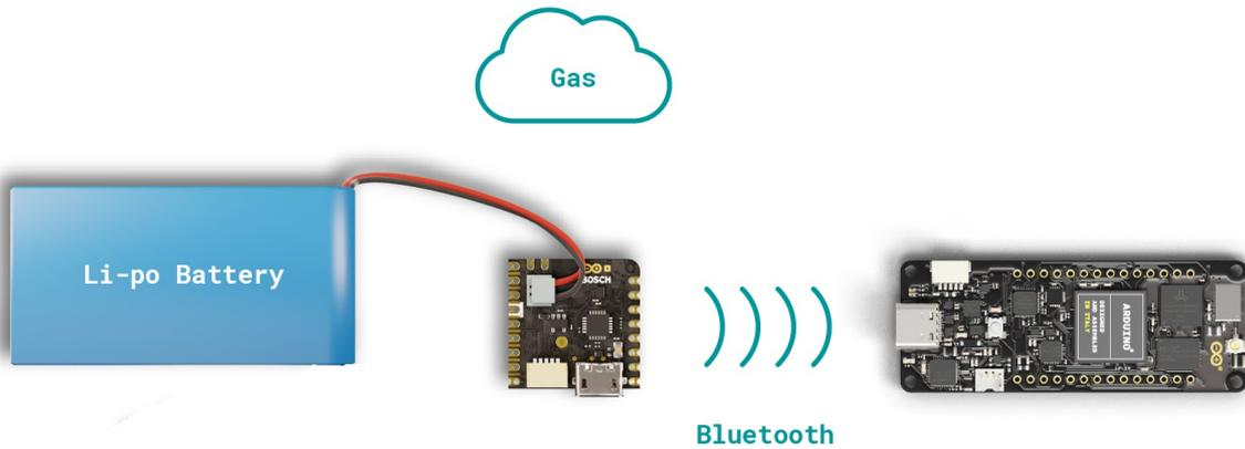
Example of a typical solution for remote environmental sensing including an Arduino® Nicla Sense ME, Arduino® Portenta H7 and LiPo battery.
