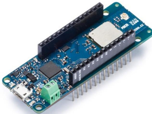
**Arduino MKR WAN 1300** has been designed to offer a practical and cost effective solution for makers seeking to add Lo-Ra connectivity to their projects with minimal previous experience in networking. It is based on the Atmel [SAM D21](#) and a Murata CMWX1ZZABZ Lo-Ra module.
