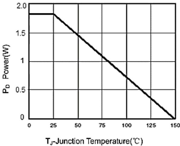
Figure 1 Power Dissipation
