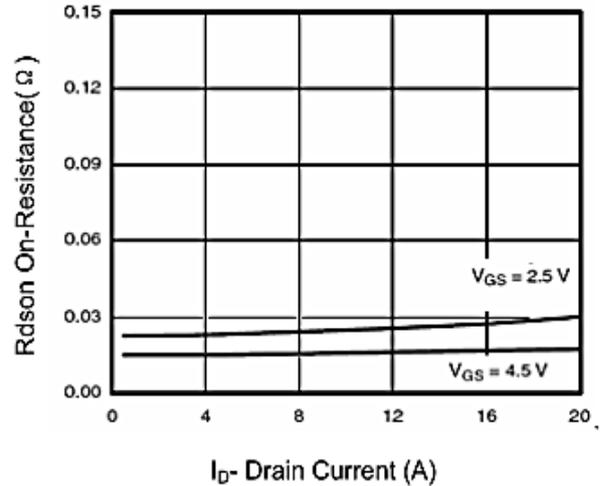
Figure 4 Drain-Source On-Resistance
