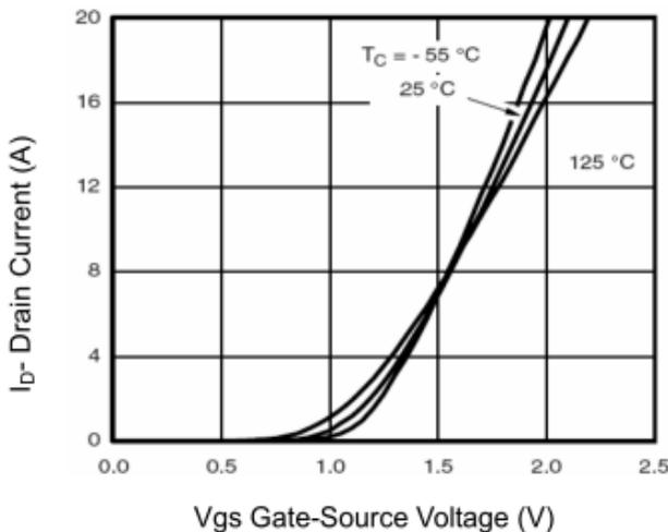
Figure 5 Transfer Characteristics
