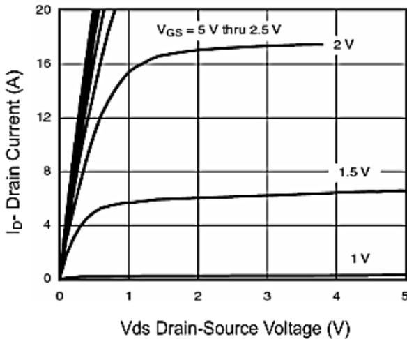
Figure 3 Output Characteristics
