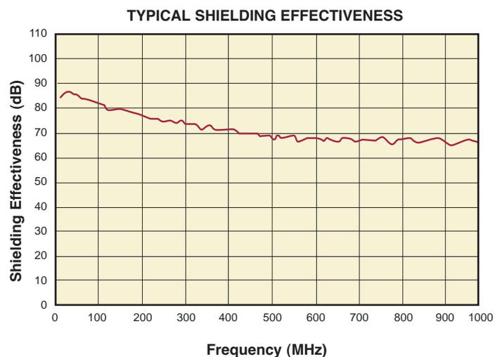
Test Methods: ASTM D-4935-89
