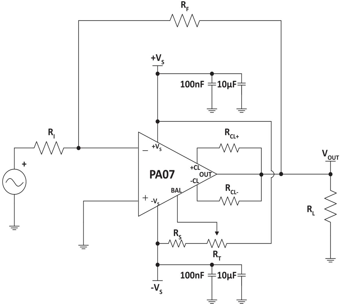
**Note:** Input offset voltage trim optional.  $R_T = 10\text{ k}\Omega\text{ MAX}$
