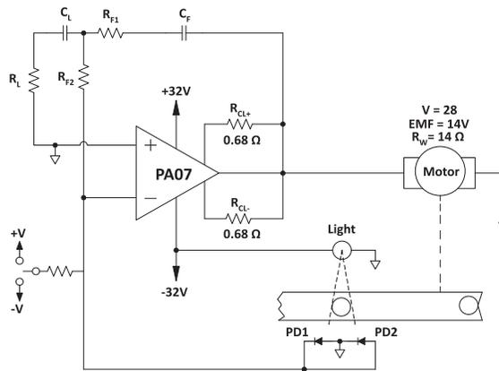
**Note:** Negates optoelectronic instabilities; Lead network minimizes overshoot; Sequential Position Control
