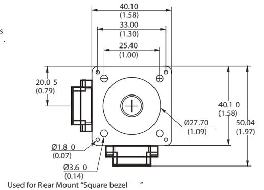
Mechanical dimensions represent a joystick with the largest potentiometer option. Potentiometer size will vary according to selected option
