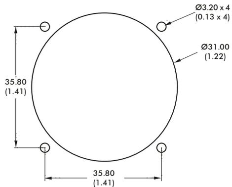
The joystick is mounted beneath the panel and the base of the boot must be brought through the panel cut-out and held in place with the circular bezel. For panel thickness of <3mm, M3 x 16 countersunk machine screws are recommended.
