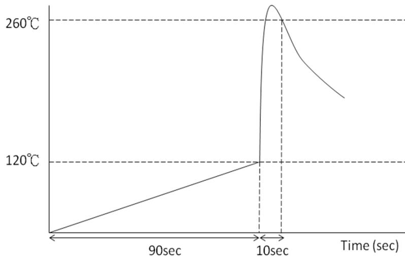
Figure 7 Flow Curve
