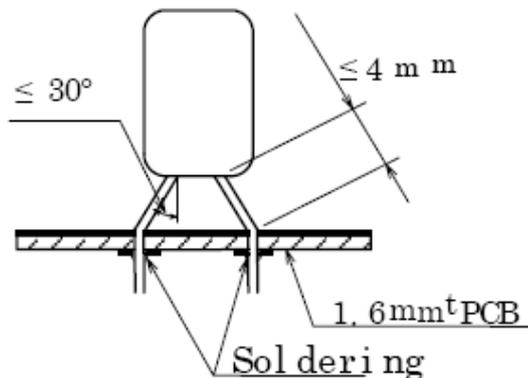
Figure 4 Vibration test
