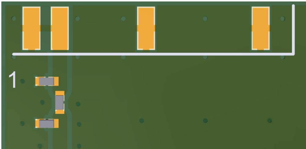
Below the footprint is shown again but without the solder mask. Pin 2 (feed) must be connected to pin 1 (GND) as shown here.
