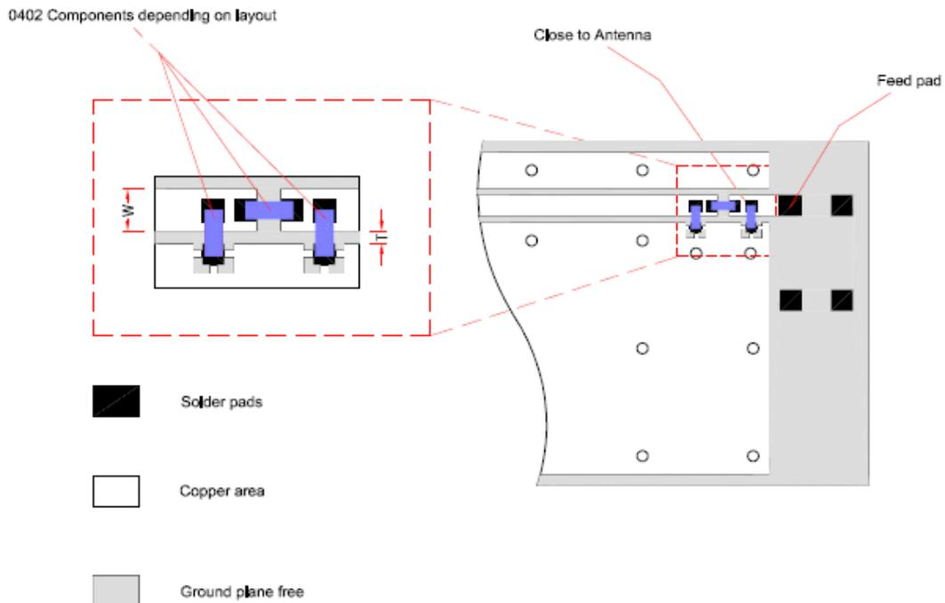
The antenna feed pad is indicated in the drawing above. Additional pads are for mechanical attachment only and should not be grounded.
