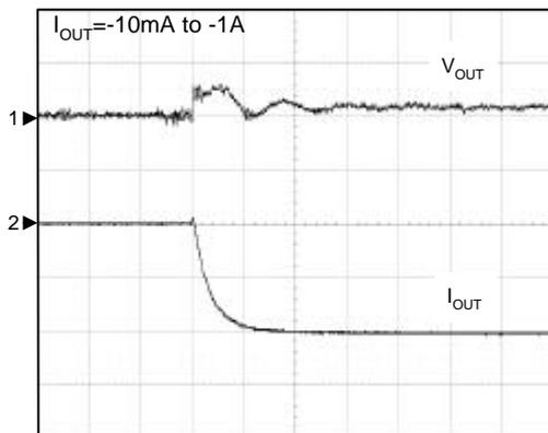
CH1:  $V_{OUT}$ , 20mV/Div, AC
