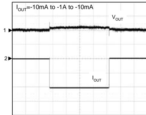
CH1:  $V_{OUT}$ , 20mV/Div, AC
