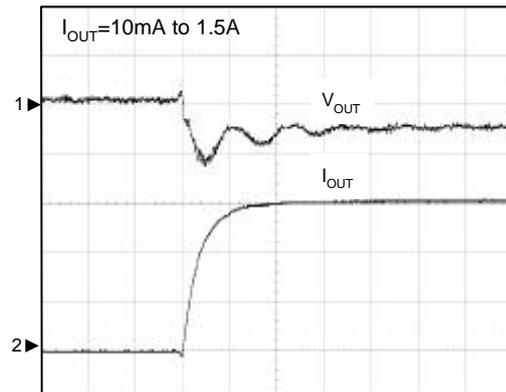
Load Transient Response ( $V_{IN} = 1.8V$ )
