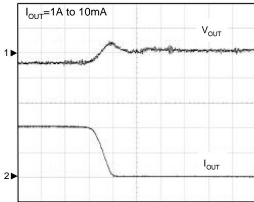
CH1:  $V_{OUT}$ , 20mV/Div, AC
