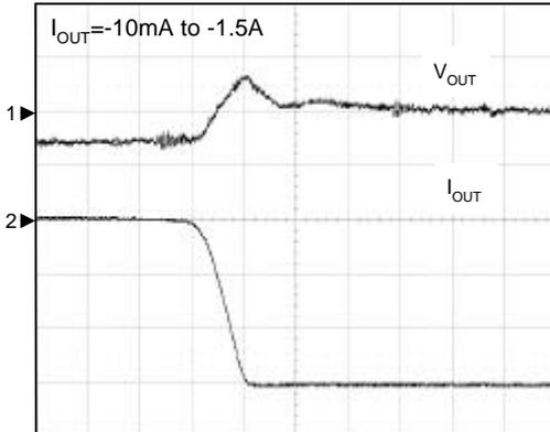
CH1:  $V_{OUT}$ , 20mV/Div, AC
