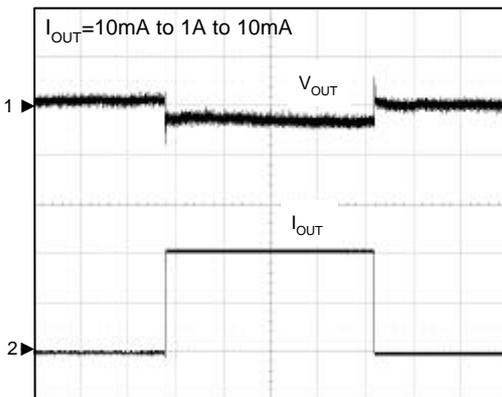
CH1:  $V_{OUT}$ , 20mV/Div, AC
