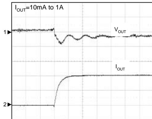
CH1:  $V_{OUT}$ , 20mV/Div, AC
