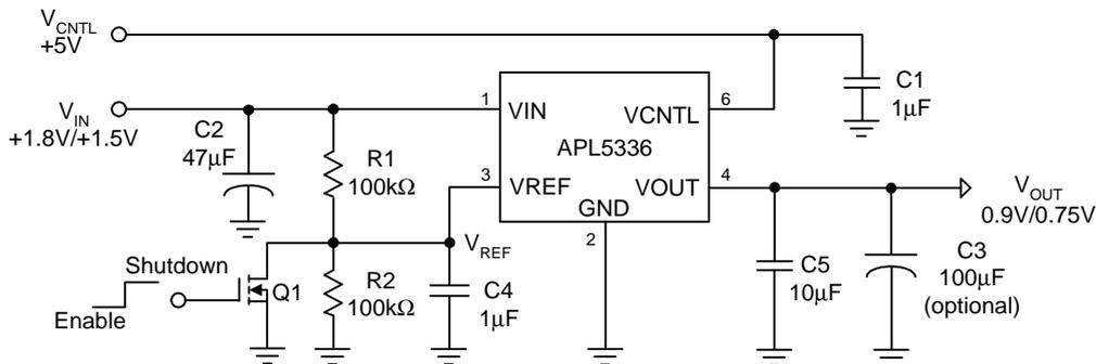
The ceramic capacitor C5 ( at least 8µF) is necessary for output stability.
