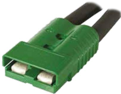
The SB® 350 is the largest connector in the series with power capabilities up to 500 amps with a 350 mcm wire. Wires ranging from 1/0 to 350 mcm (53.5 to 185 mm<sup>2</sup>) fit into the one piece housing available in standard PC or a chemical resistant PBT/PC blend. Silver plated wire or busbar contacts minimize electrical resistance while offering supreme durability and reliability.
