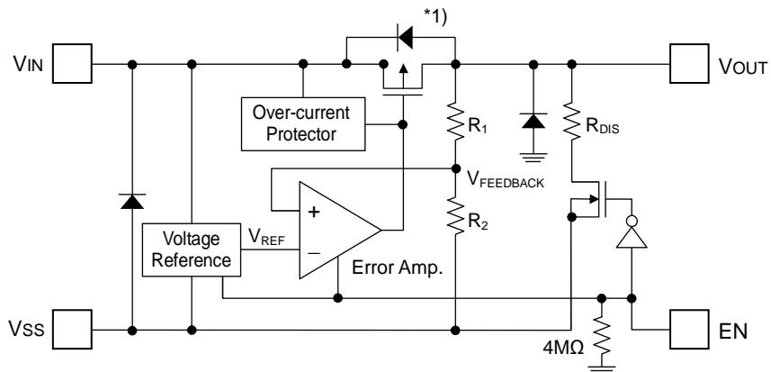
By the error amplifier, the reference voltage ( $V_{REF}$ ) is compared with  $V_{FEEDBACK}$  which is divided by feedback resistors  $R_1$  and  $R_2$ . It supplies the output transistor (see note \*1) to keep a stabilized output voltage against with any fluctuation of input voltage by negative feedback system.
