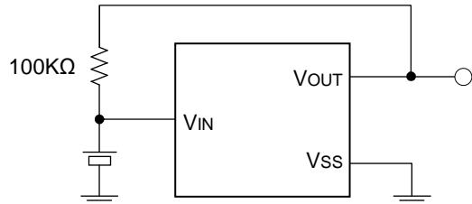
**BLOCK DIAGRAM**● **CMOS output**
