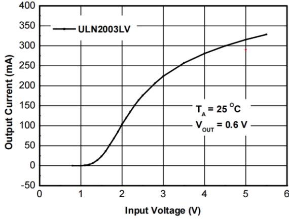
Output Current vs. Input Voltage (All Darlings in Parallel)
