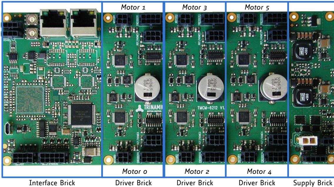
Figure 5.1 different bricks used for the TMCM-6212 / TMCM-6213
