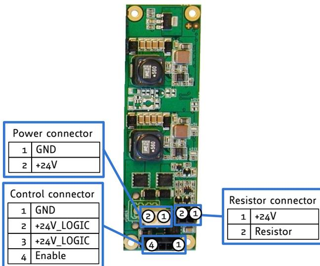
Figure 5.5: TMCM-6212 + TMCM-6213 Power supply Brick
