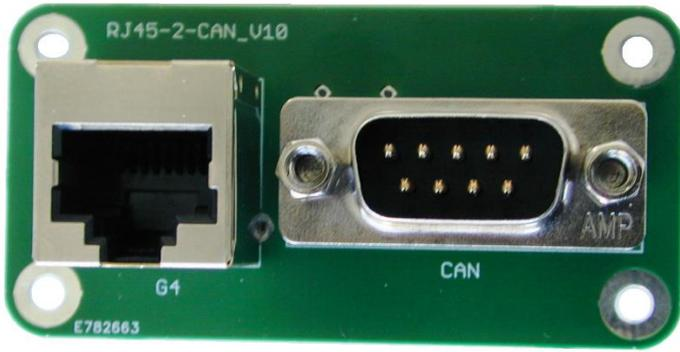
Figure 5.6: RJ45-2-DSUB PCB top view
