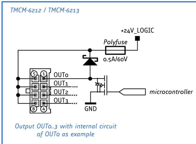
Figure 5.8: General purpose output – internal circuit (simplified)
