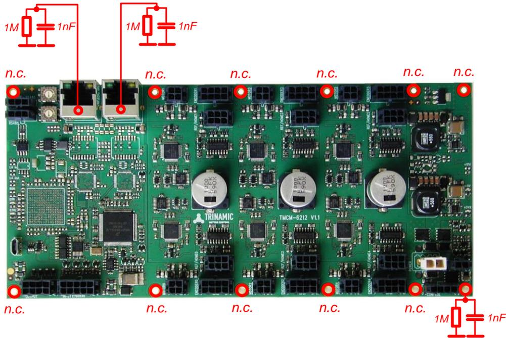
**Figure 4.2 TMC6212 / TMC6213 mounting hole connections**
