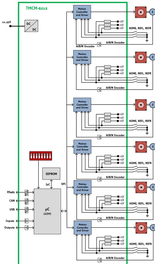
Figure 10.1 Main parts of the TMCM-6212
