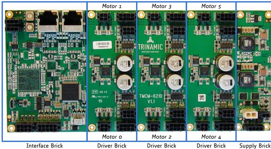
Figure 5.1 different bricks used for the TMCM-6210 / TMCM-6211
