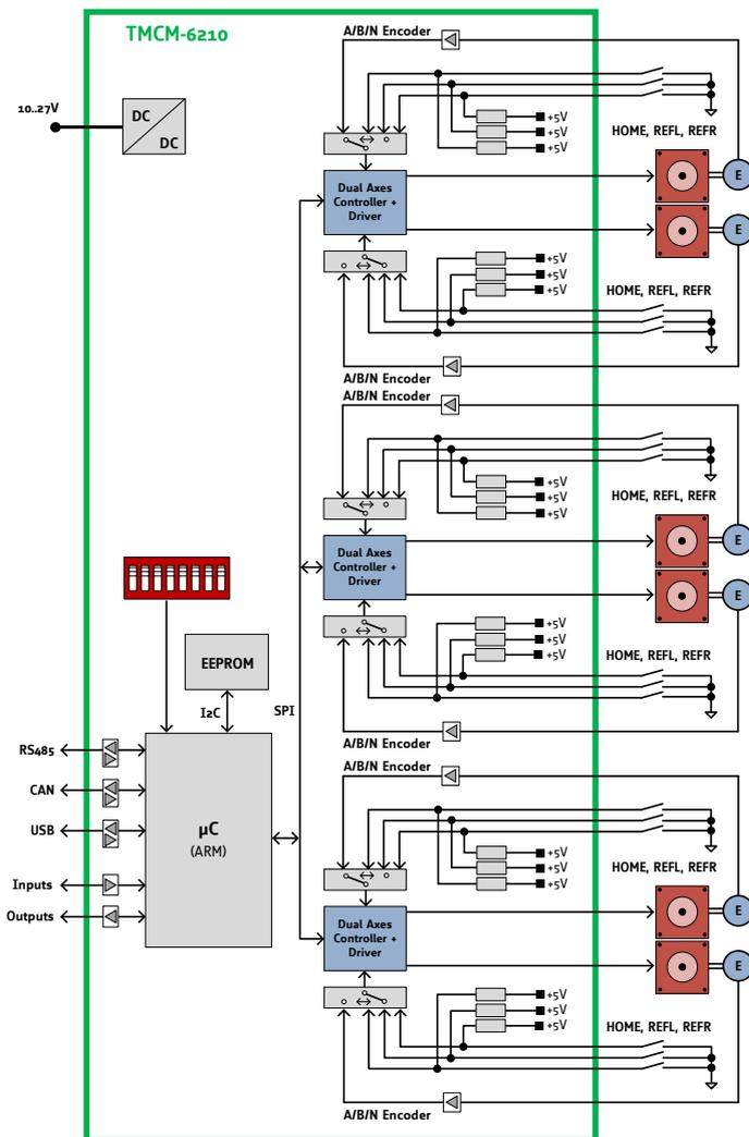
Figure 10.1 Main parts of the TMCM-6210
