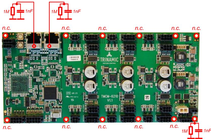
**Figure 4.2 TMCM-6210 / TMCM-6211 mounting hole connections**
