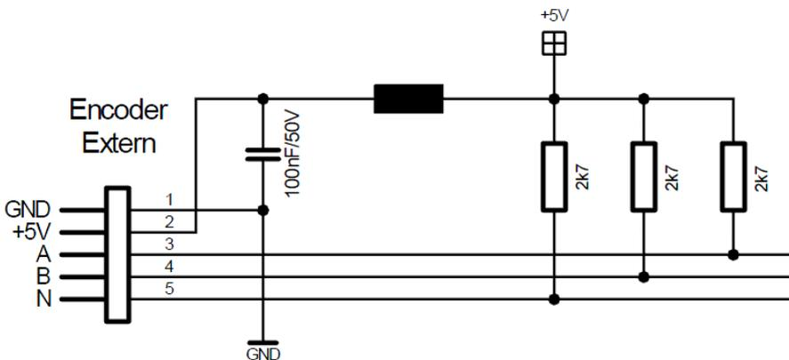
Figure 4.4: Encoder input circuit
