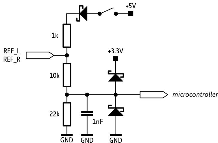
Figure 3.9 Reference switch input circuit (simplified diagram)
