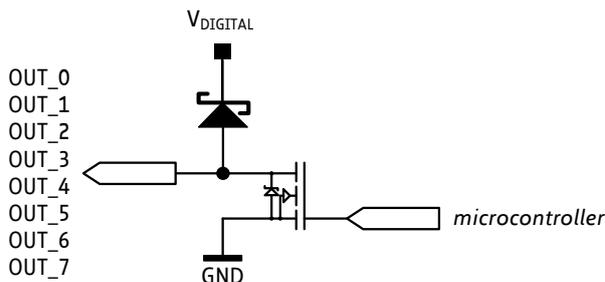
Figure 3.12 General purpose output (open-drain with freewheeling diode)
