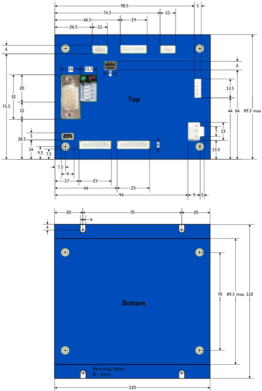
Figure 3.1 Dimensions of TMCM-1311 (all values in mm).
