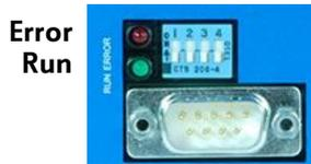
**Figure 4.1 On-board LEDs**
