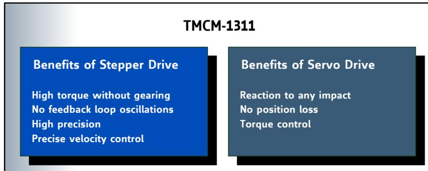
Figure 1.1 TMC-1311 characteristics in closed loop mode
