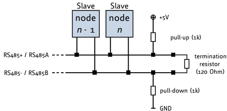
**Figure 3.5 RS485 bus lines with resistor network**
