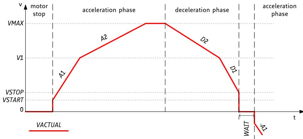
Figure 5: Typical motion profile with TRINAMIC's sixPoint motion controller
