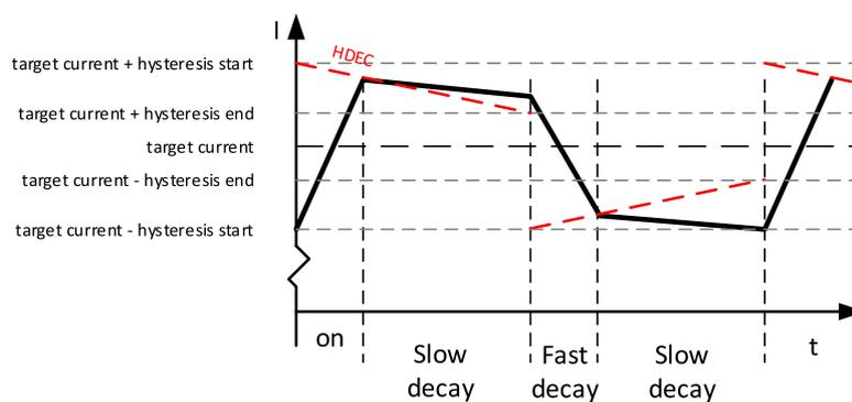
Figure 2: spreadCycle principle
