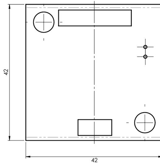
Figure 6: TMCM-1270 top view mechanical dimensions
