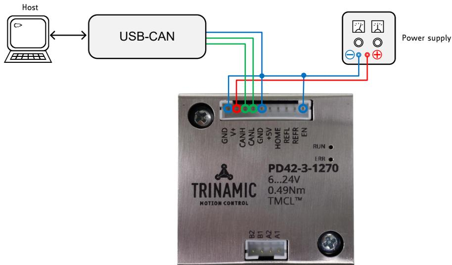
Figure 11: Typical application scenario for remote control of TMCM-1270
