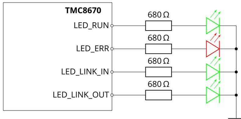
Figure 8: Status LED circuit
