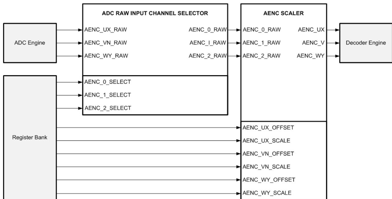
Figure 18: Analog Encoder (AENC) Selector & Scaler w/ Offset Correction
