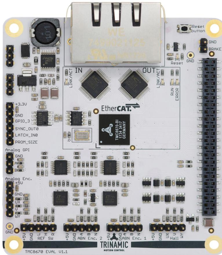
Figure 3: TMC8670 Evaluation Board
