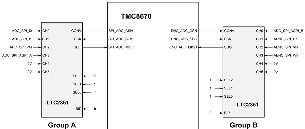
Figure 16: TMC8670 configuration for LTC2351 SPI ADCs
