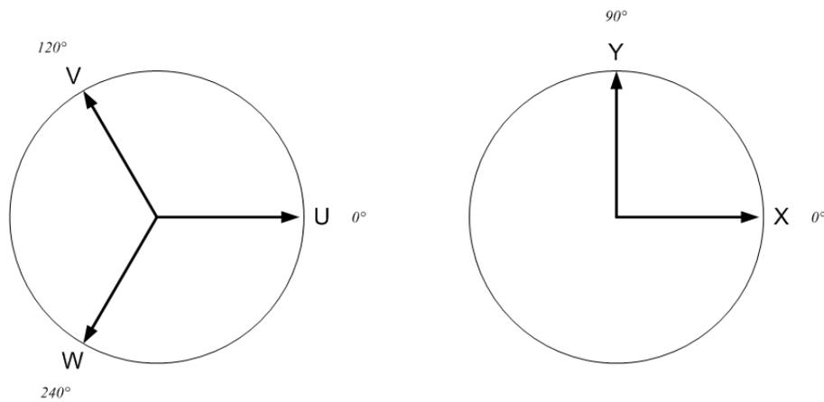
Figure 24: Orientations UVW (FOC3) and XY (FOC2)
