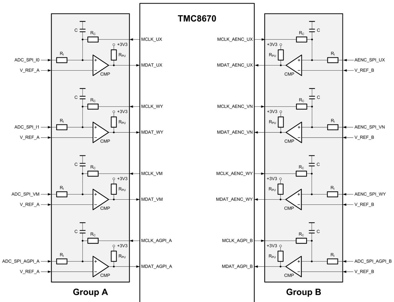
Figure 15: TMC8670 Delta Sigma ADC Configuration
