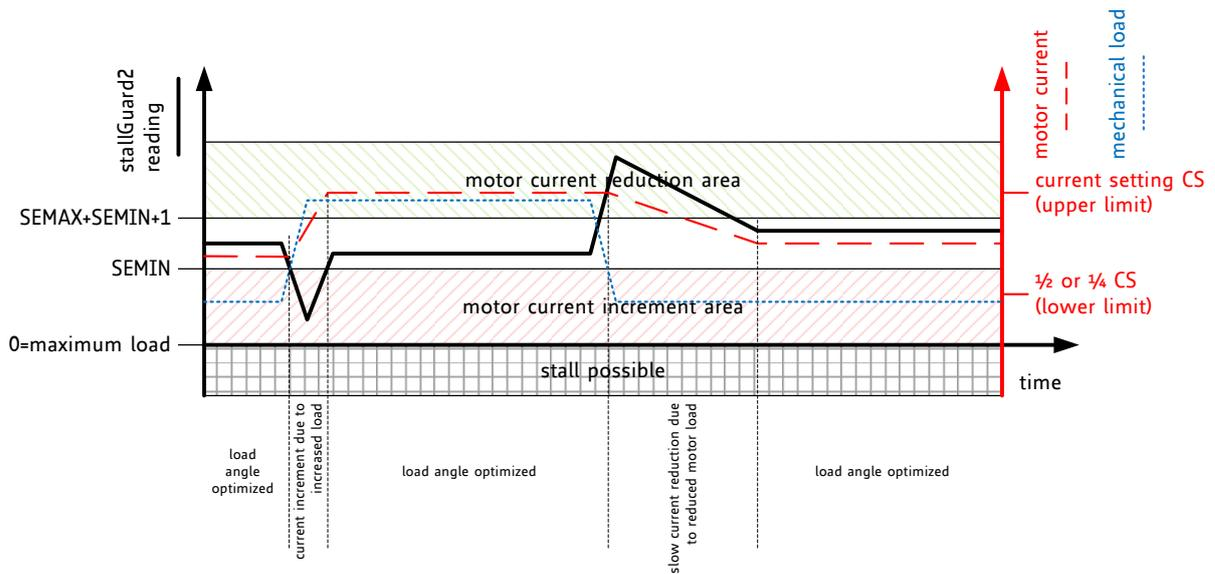
**Figure 6.2 CoolStep adapts motor current to the load.**
