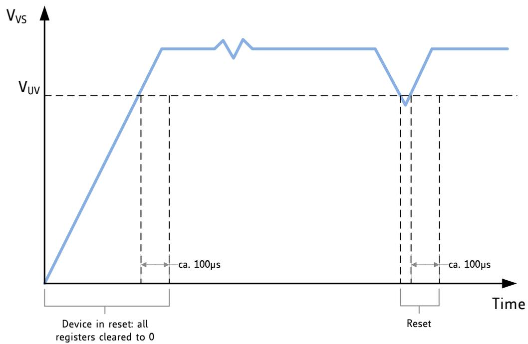
**Figure 12.2 Undervoltage reset timing****Note**
