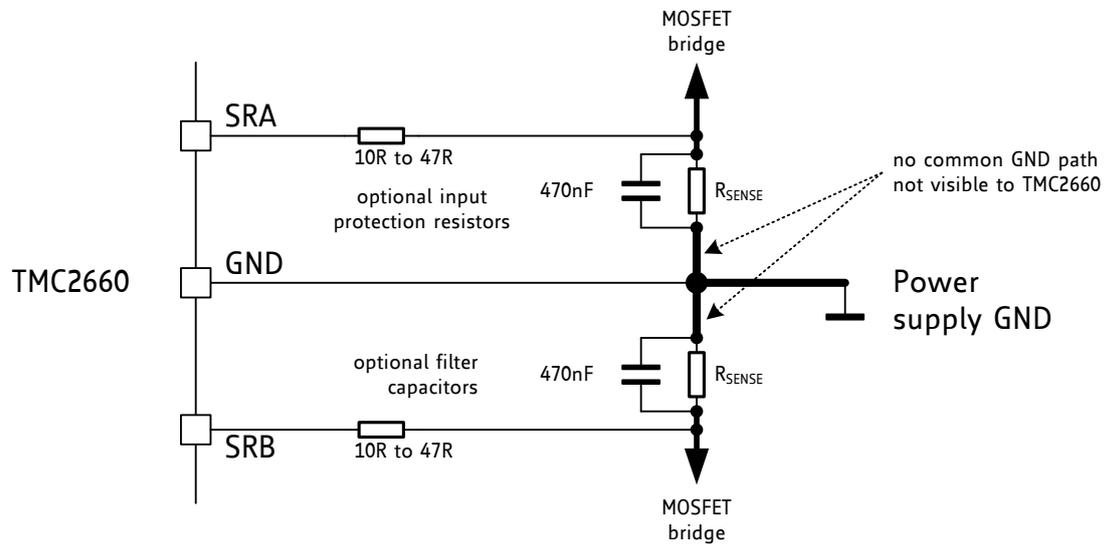
**Figure 9.1** Sense resistor grounding and protection components
