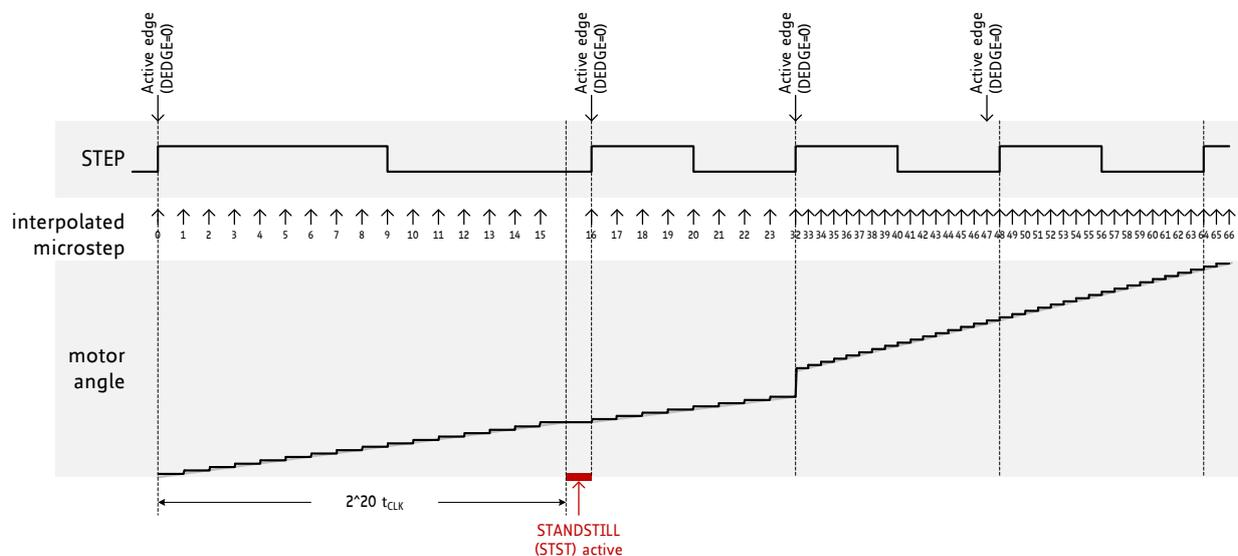
Figure 8.3 MicroPlyer microstep interpolation with rising STEP frequency.
