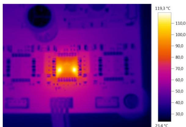
Figure 19.1 TMC2660 operating at 2.3A RMS (3.2A peak) on a 50cm<sup>2</sup> sized board
