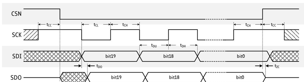
**Figure 7.1** SPI Timing
