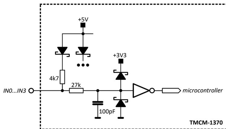
Figure 4: Digital inputs HOME, STOP\_L, STOP\_R and /ENABLE
