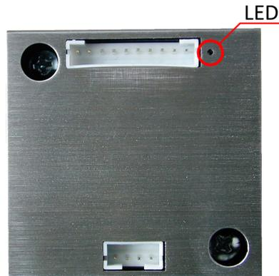
Figure 3: PD42-x-1370 LEDs
