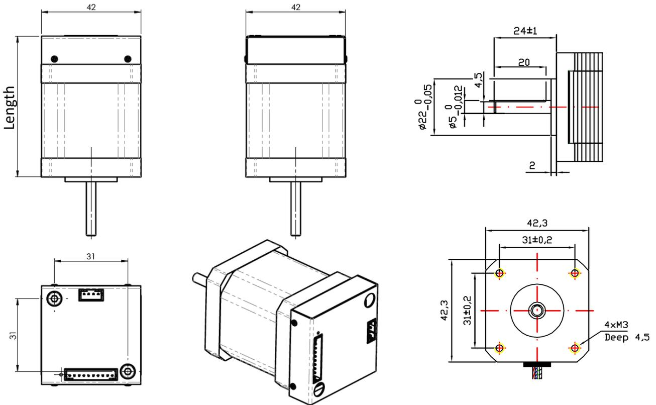
Figure 1: PD42-x-1370 with different NEMA17 / 42mm stepper motors (all dimensions in mm)
