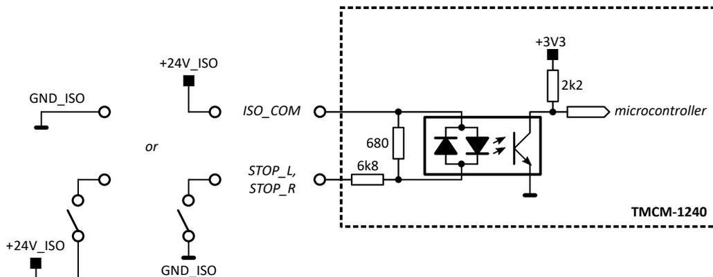
Figure 7: Stop switch inputs
