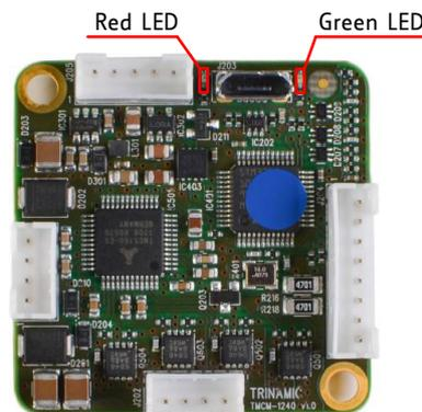
Figure 3: PD42-x-1240 LEDs
