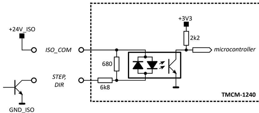
Figure 9: Step/Direction input
