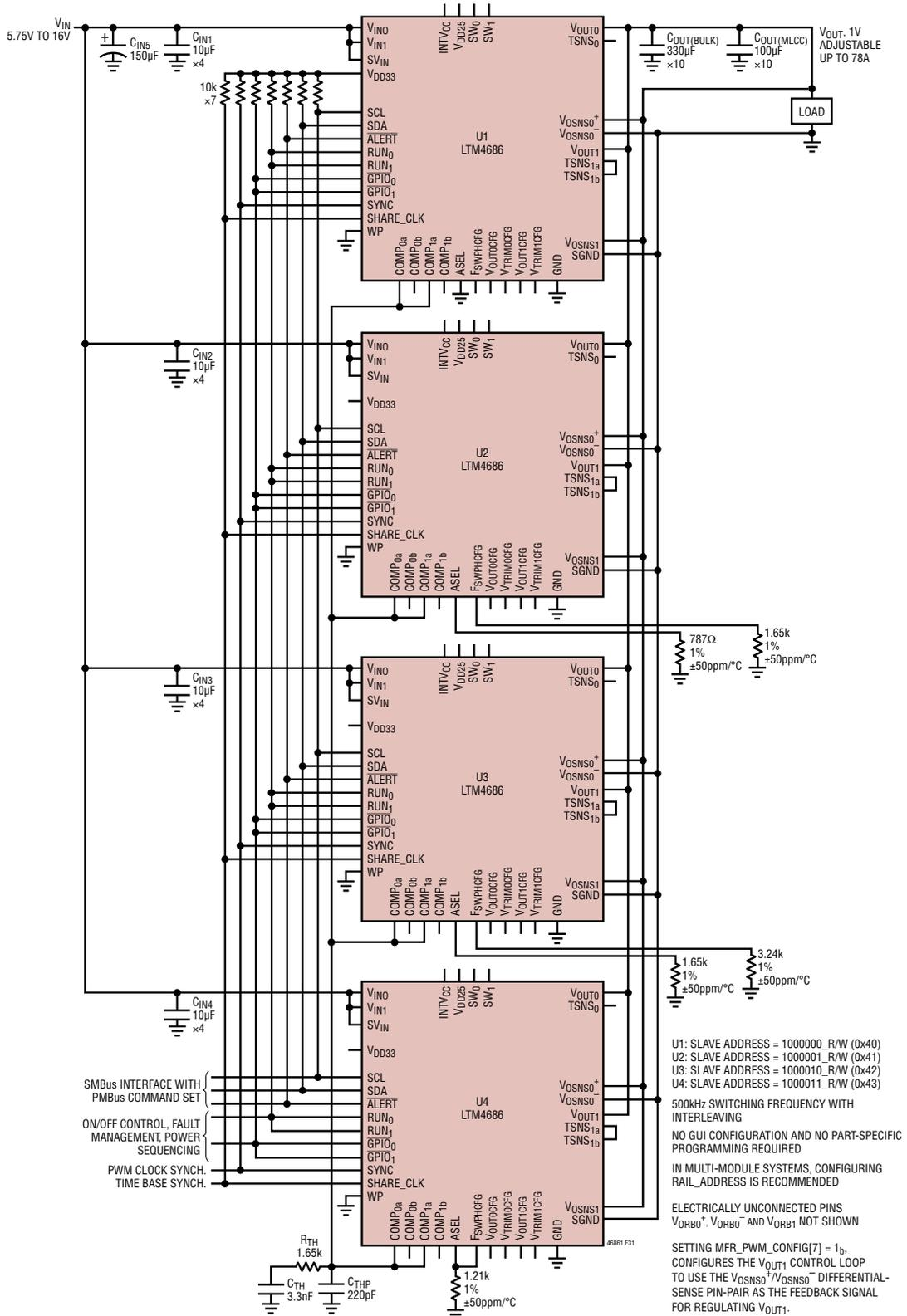
Figure 31. Four Paralleled LTM4686 Producing 1V<sub>OUT</sub> at Up to 78A. Integrated Power System Management Features Accessible Over 2-Wire I<sup>2</sup>C/SMBus/PMBus Serial Interface. Evaluated on DC1989B-C, Custom-Stuffed with LTM4686 Modules
