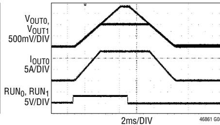
FIGURE 61 CIRCUIT AT  $12\text{V}_{\text{IN}}$ . 100mΩ LOAD ON V<sub>OUT0</sub>. NO LOAD ON V<sub>OUT1</sub>. TON\_RISE<sub>0</sub> = 3ms, TON\_RISE<sub>1</sub> = 5.297ms, TOFF\_DELAY<sub>1</sub> = 0ms, TOFF\_DELAY<sub>0</sub> = 2.43ms, TOFF\_FALL<sub>1</sub> = 5.328ms, TOFF\_FALL<sub>0</sub> = 3ms, ON\_OFF\_CONFIG<sub>n</sub> = 0x1E
