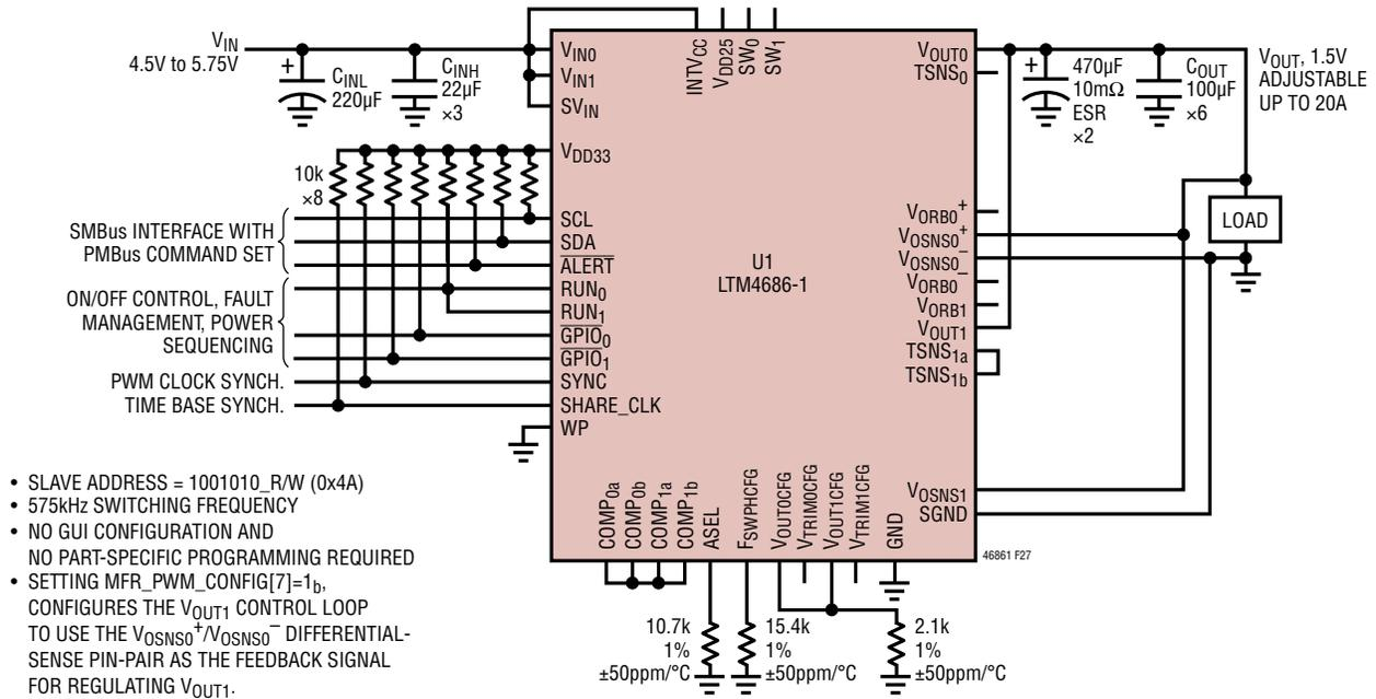
Figure 27. 20A, 1.5V Output DC/DC  $\mu$ Module Regulator with I<sup>2</sup>C/SMBus/PMBus Serial Interface
