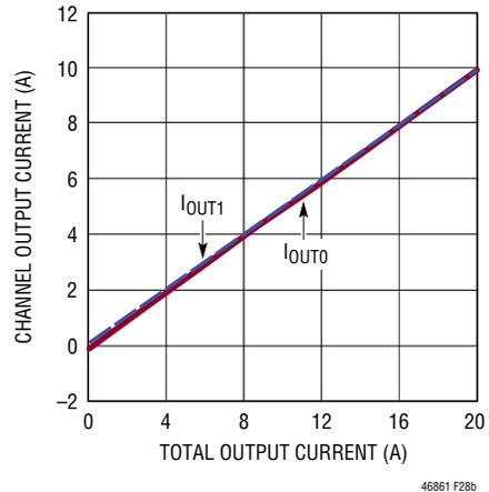
(28b) 12V<sub>IN</sub>, Figure 27 Circuit with U1 Installed with LTM4686, INTV<sub>CC</sub> Open and V<sub>OUT</sub> Commanded to 1V
