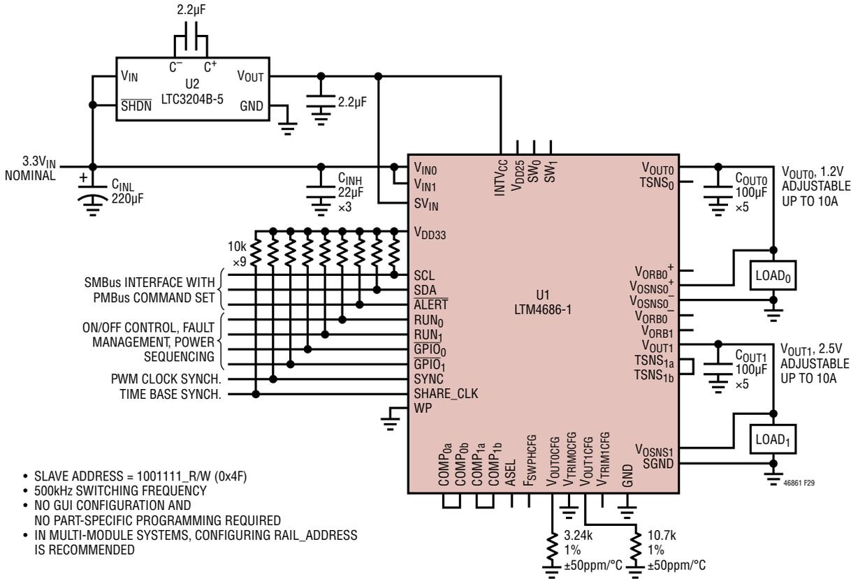
Figure 29. 10A, 1.2V and 2.5V Outputs Generated from 3.3V Power Input and Providing I<sup>2</sup>C/SMBus/PMBus Serial Interface
