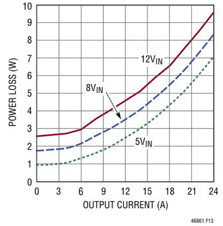
Figure 13. 3.3V<sub>OUT</sub> Power Loss Curve
