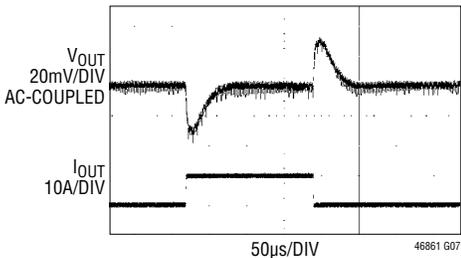
FIGURE 27 CIRCUIT AT  $5\text{V}_{\text{IN}}$ . VOUT\_COMMAND<sub>n</sub> SET TO 1.000V. 10A TO 20A LOAD STEP AT 10A/μs
