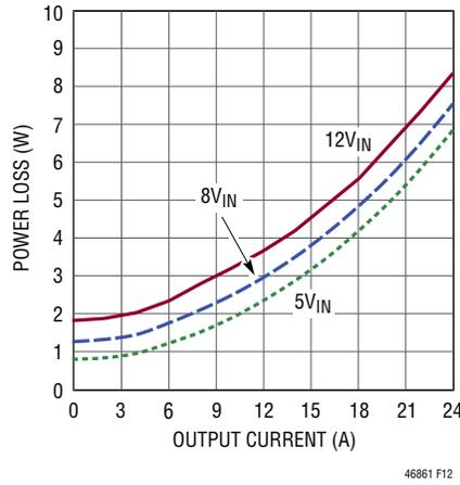
Figure 12. 1.8V<sub>OUT</sub> Power Loss Curve
