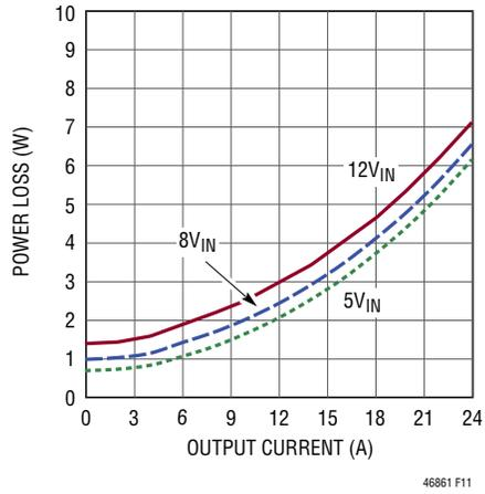
Figure 11. 1V<sub>OUT</sub> Power Loss Curve
