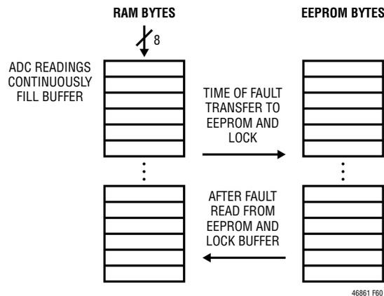
Figure 60. Fault Log Conceptual Diagram
