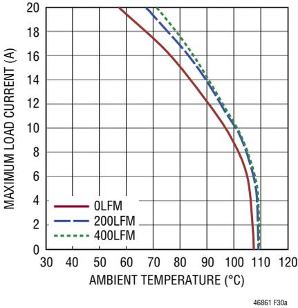
(30a) Single 20A, 1V<sub>OUT</sub>, No Heat Sink
