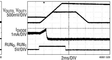
FIGURE 61 CIRCUIT AT  $12\text{V}_{\text{IN}}$ . 100mΩ LOAD ON V<sub>OUT0</sub>. 500Ω ON V<sub>OUT1</sub>. V<sub>OUT1</sub> PRE-BIASED THROUGH A DIODE. TON\_RISE<sub>0</sub> = 3ms, TON\_RISE<sub>1</sub> = 5.297ms, TOFF\_DELAY<sub>1</sub> = 0ms, TOFF\_DELAY<sub>0</sub> = 2.43ms, TOFF\_FALL<sub>1</sub> = 5.328ms, TOFF\_FALL<sub>0</sub> = 3ms, ON\_OFF\_CONFIG<sub>1</sub> = 0x1F, ON\_OFF\_CONFIG<sub>0</sub> = 0x1E
