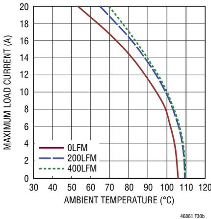
(30b) Single 20A, 1.8V<sub>OUT</sub>, No Heat Sink
