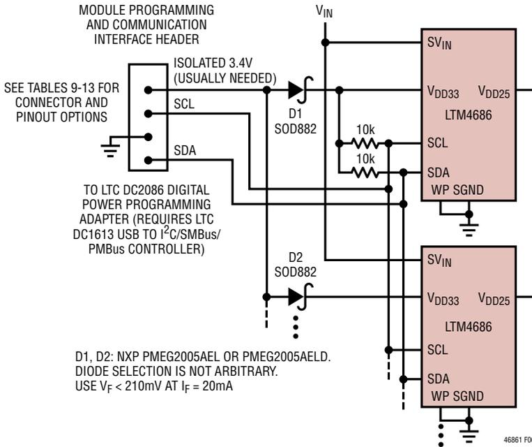
Figure 6. Circuit Suitable for Programming EEPROM/NVM of LTM4686 and Other ADI PSM Modules/ICs in Vast Systems, Even When  $V_{IN}$  Power is Absent,  $T_A > 20^{\circ}C$  and  $T_J < 85^{\circ}C$
