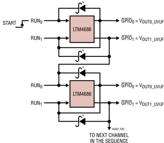
NOTE: RESISTOR OR RC PULL-UPS ON  $\text{RUN}_n$  AND  $\overline{\text{GPIO}}_n$  PINS NOT SHOWN
