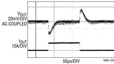
FIGURE 27 CIRCUIT AT  $12\text{V}_{\text{IN}}$ . INTV<sub>CC</sub> PIN OPEN CIRCUIT AND VOUT\_COMMAND<sub>n</sub> SET TO 1.000V. 10A TO 20A LOAD STEP AT 10A/μs
