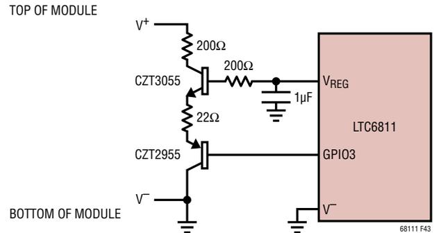
Figure 43. 200mA Module Balancer
