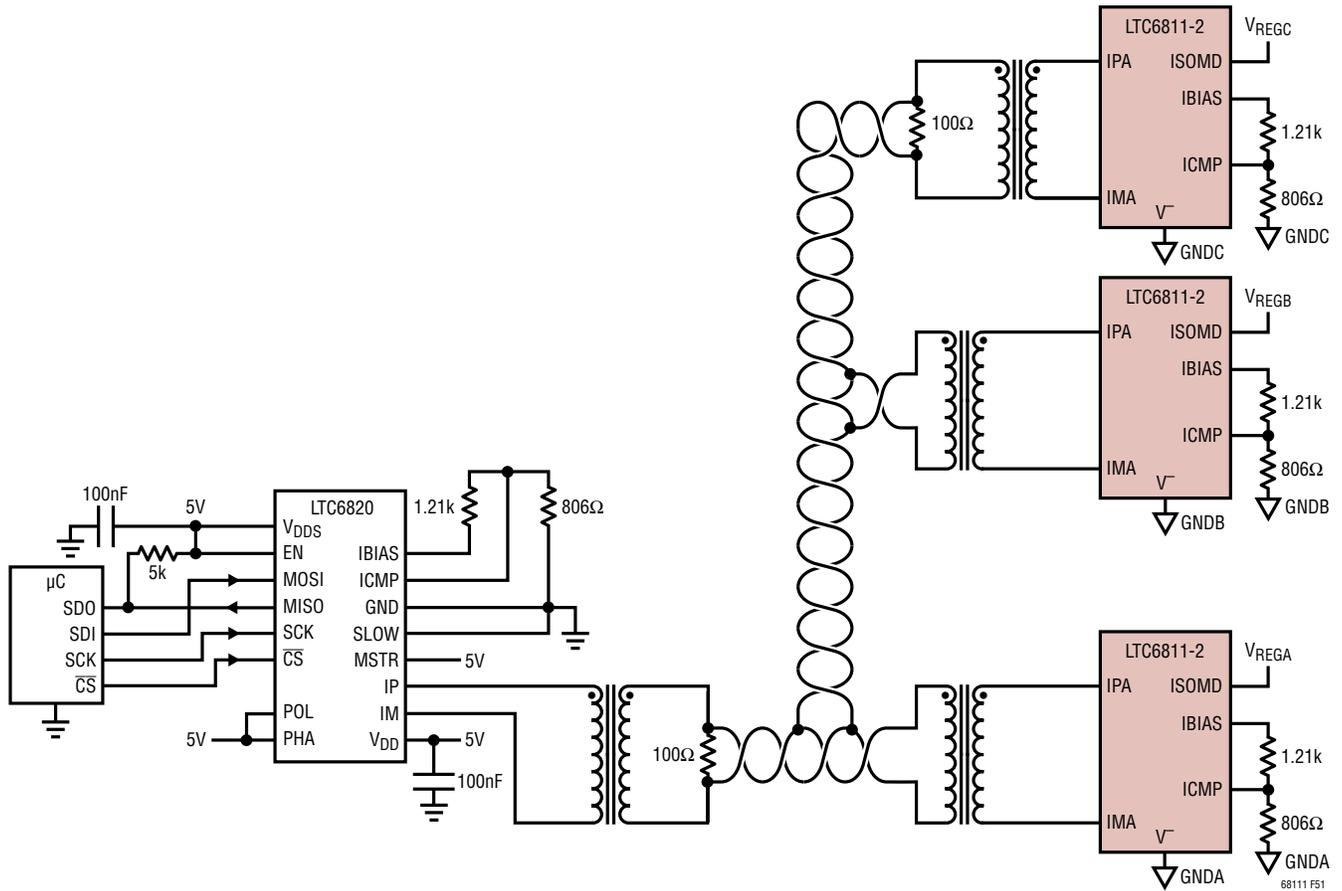
Figure 51. Connecting the LTC6811-2 in a Multi-Drop Configuration
