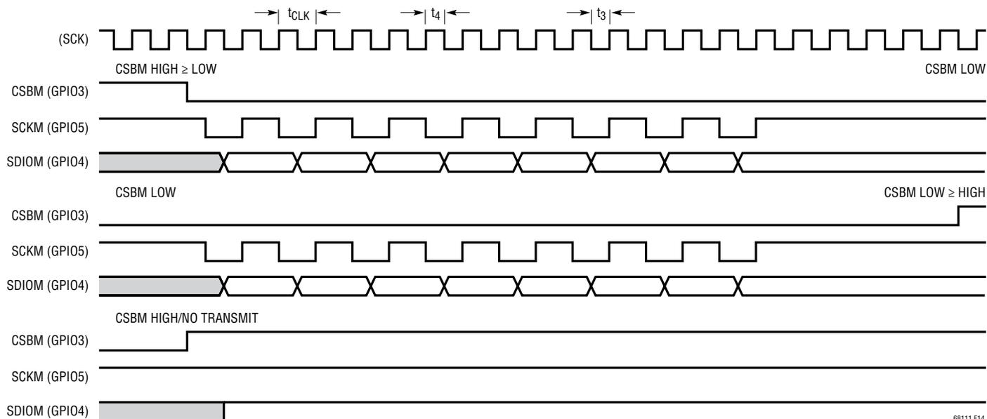
Figure 14. STCOMM Timing Diagram for a SPI Master
