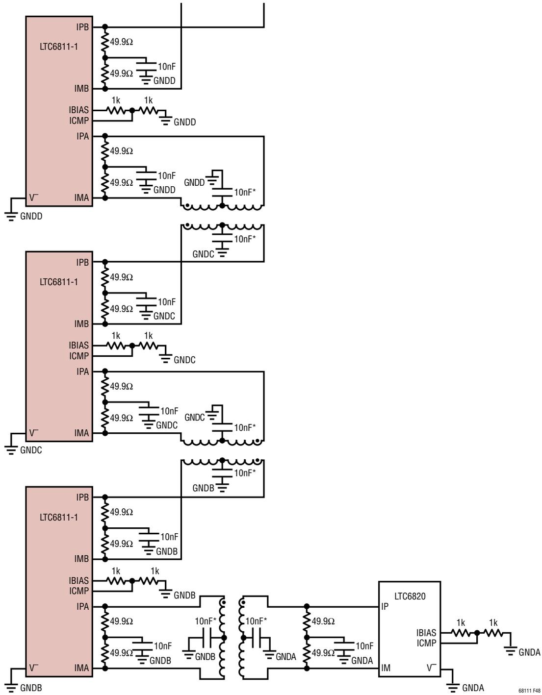
Figure 48. Daisy Chain Interface Components on Single Board
