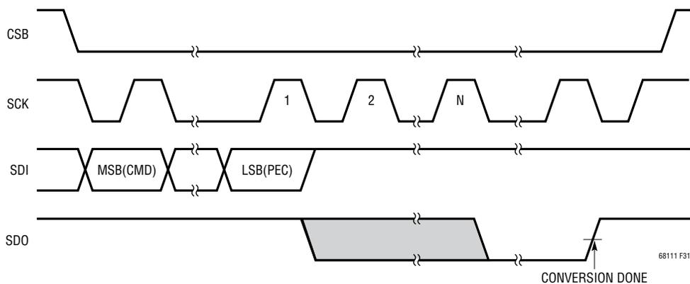
Figure 31. SDO Polling Using PLADC Command (Daisy-Chain Configuration)
