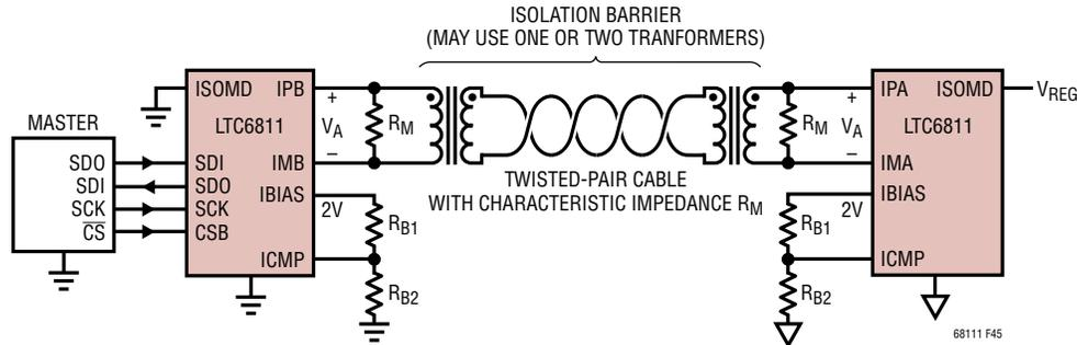
Figure 45. isoSPI Circuit
