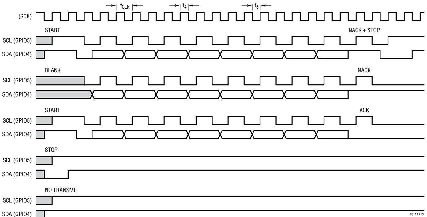
Figure 13. STCOMM Timing Diagram for an I<sup>2</sup>C Master
