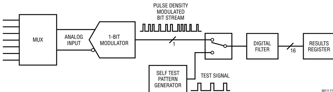
Figure 10. Operation of LTC6811 ADC Self Test
