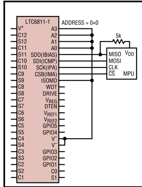
Figure 23. Single Device LTC6811-2 Using 4-Wire Port A
