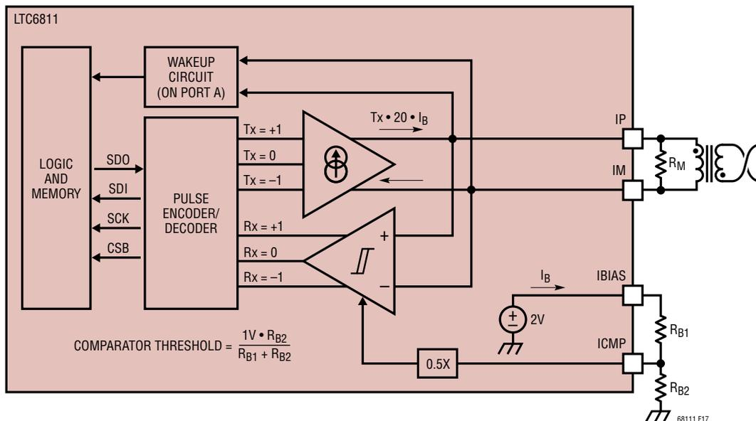
Figure 17. isoSPI Interface
