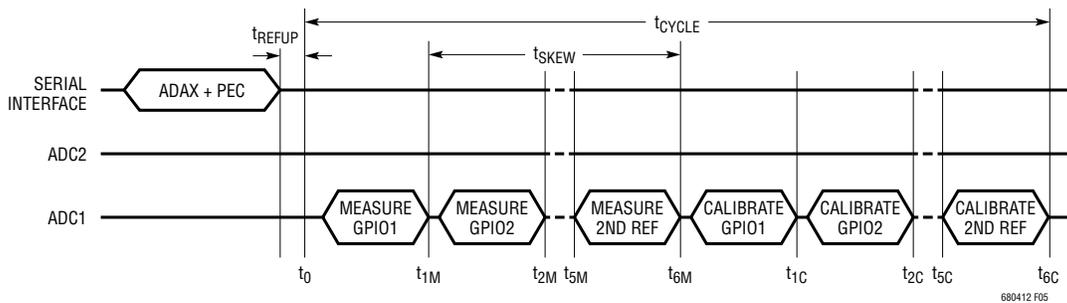
Figure 5. Timing for ADAX Command Measuring All GPIOs and 2<sup>nd</sup> Reference
