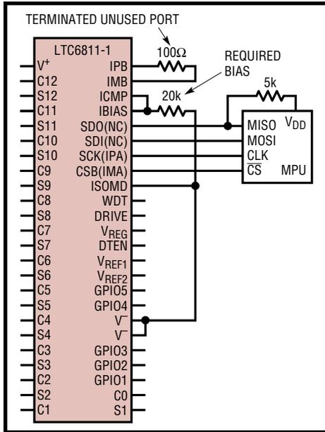
Figure 22. Single Device LTC6811-1 Using 4-Wire Port A
