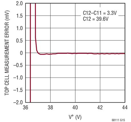
**Measurement Error vs Common Mode Voltage**
