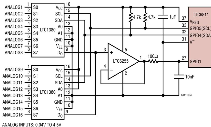
Figure 58. MUX Circuit Supports Sixteen Additional Analog Measurements
