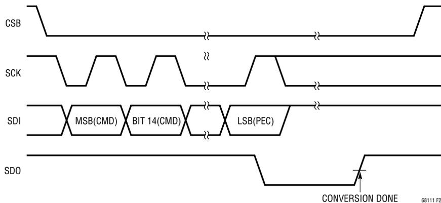
Figure 29. SDO Polling Using PLADC Command (Parallel Configuration)
