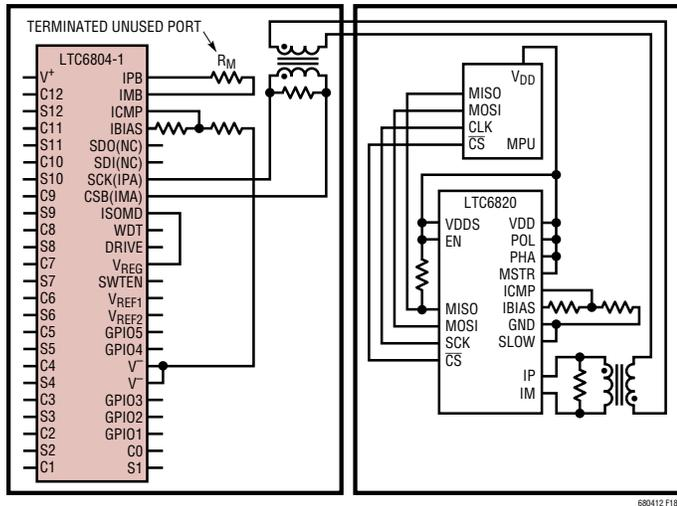
Figure 18a. Single-Device LTC6804-1 Using 2-Wire Port A
