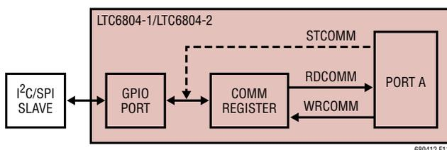
**Figure 11. LTC6804 I<sup>2</sup>C/SPI Master Using GPIOs**
