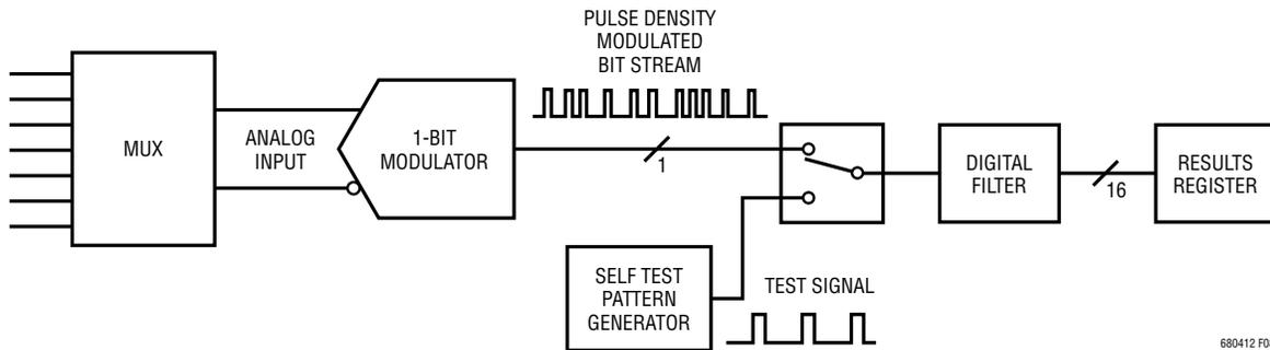
Figure 8. Operation of LTC6804 ADC Self Test
