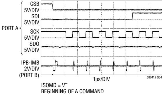
**Write Command to a Daisy-Chained Device (ISOMD = 1)**
