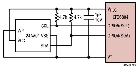
Figure 25. Connecting I<sup>2</sup>C EEPROM to LTC6804 GPIO Pins
