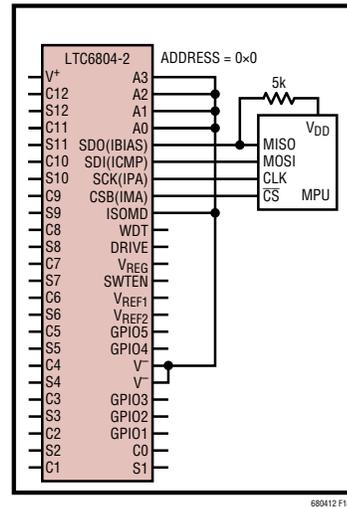
Figure 18d. Single-Device LTC6804-2 Using 4-Wire Port A
