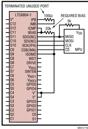
Figure 18c. Single-Device LTC6804-1 Using 4-Wire Port A
