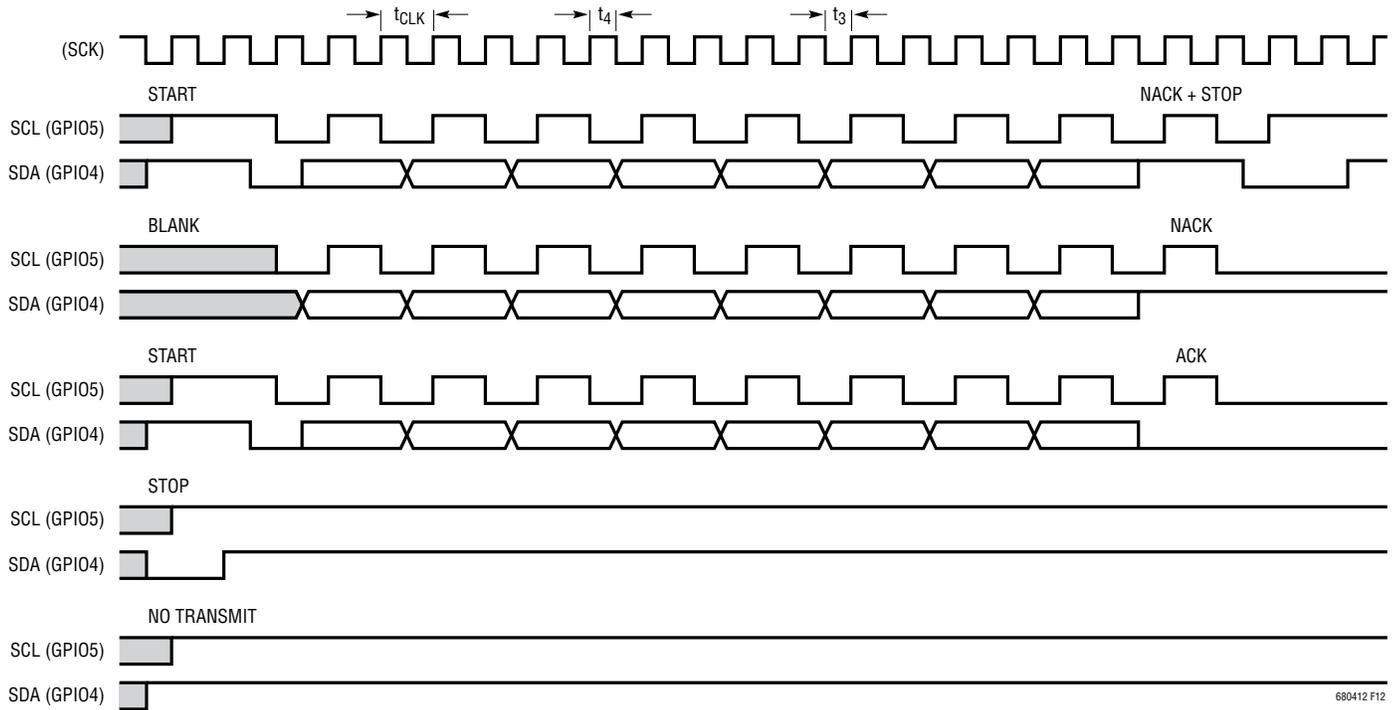
Figure 12. STCOMM Timing Diagram for an I<sup>2</sup>C Master
