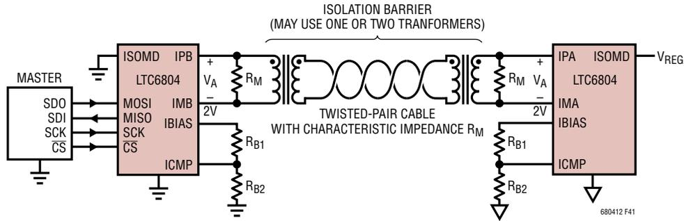
Figure 41. isoSPI Circuit
