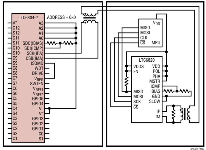
Figure 18b. Single-Device LTC6804-2 Using 2-Wire Port A
