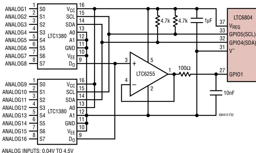
Figure 32. MUX Circuit Supports Sixteen Additional Analog Measurements
