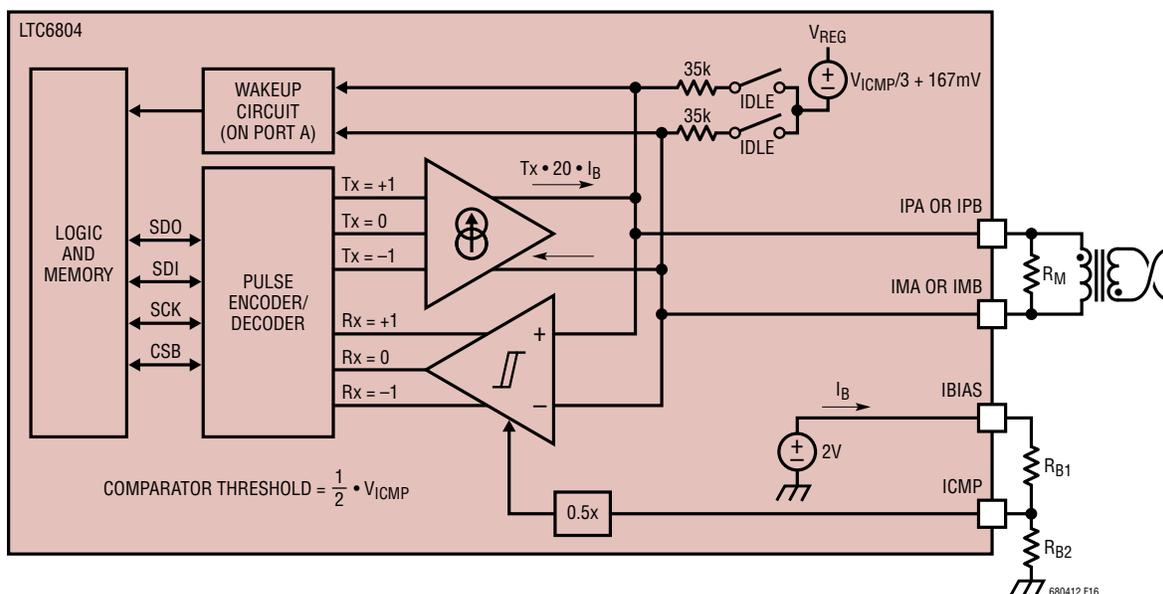
Figure 16. isoSPI Interface
