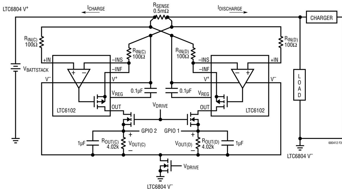
$$\text{DISCHARGING: } V_{OUT(D)} = I_{DISCHARGE} \cdot R_{SENSE} \left( \frac{R_{OUT(D)}}{R_{IN(D)}} \right) \text{ WHEN } I_{DISCHARGE} \geq 0$$
