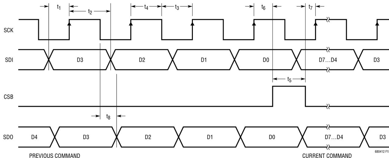
Figure 15. Timing Diagram of 4-Wire Serial Peripheral Interface
