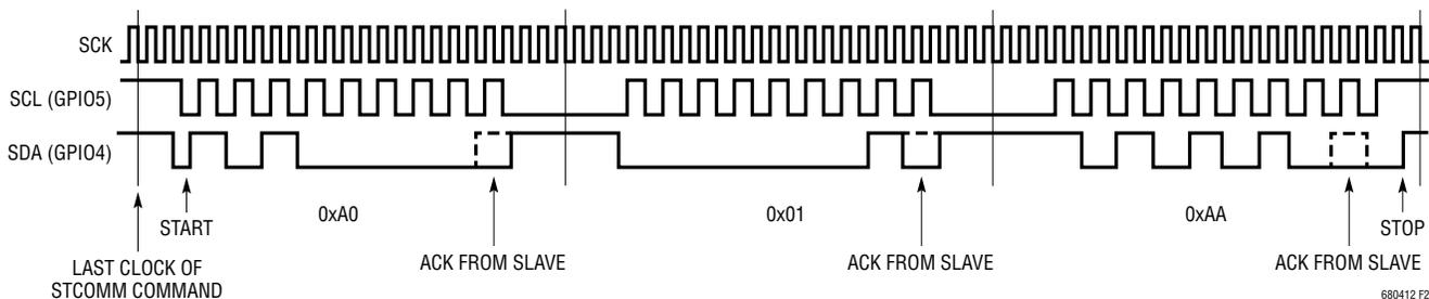
Figure 26. LTC6804 I<sup>2</sup>C Communication Example
