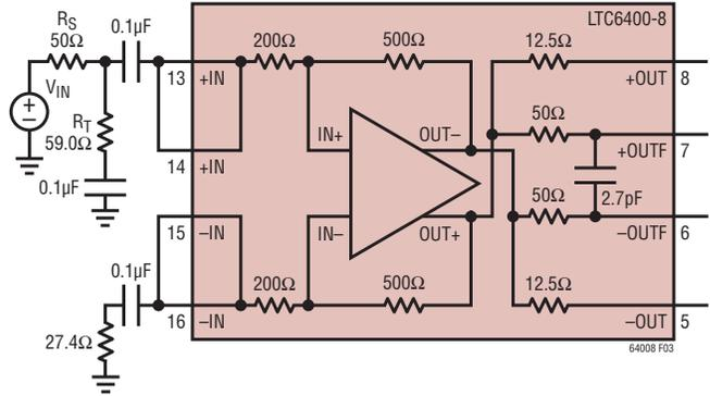
Figure 3. Input Termination for Single-Ended 50Ω Input Impedance
