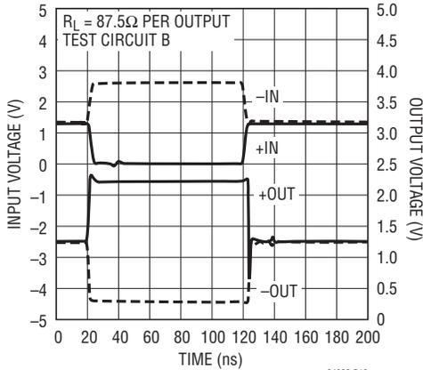
**1% Settling Time for 2V Output Step**
