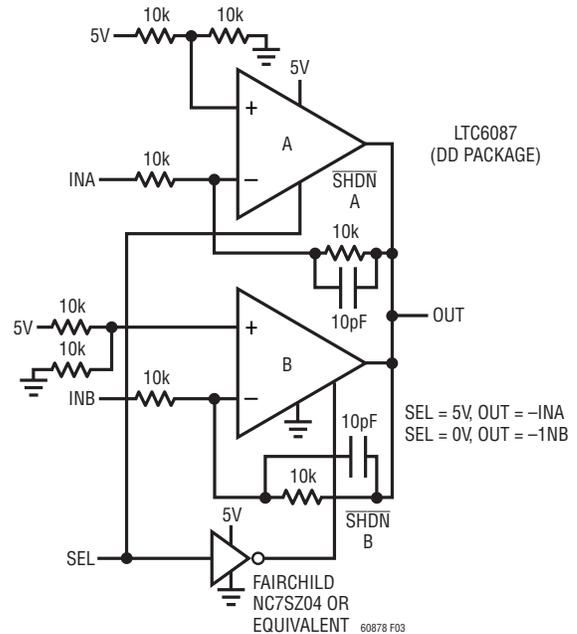
Figure 3. Inverting Amplifier with Muxed Output
