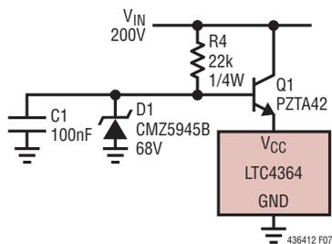
Figure 7. Buffering  $V_{CC}$  to Extend Input Supply Range
