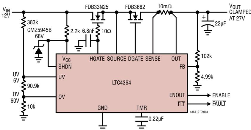
**Overvoltage Protector Regulates Output at 27V During Input Transient**
