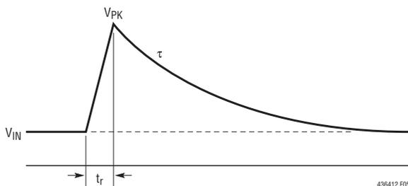
Figure 5. Prototypical Transient Waveform
