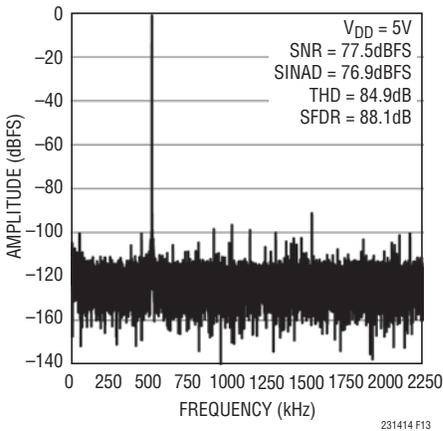
Figure 13. 32k Point FFT of the LTC2314-14 at  $f_{IN} = 500$  kHz
