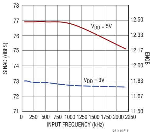
Figure 14. LTC2314-14 ENOB/SINAD vs  $f_{IN}$
