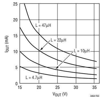
**Figure 3. Maximum Output Current**
