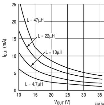
**Figure 2. Maximum Output Current**
