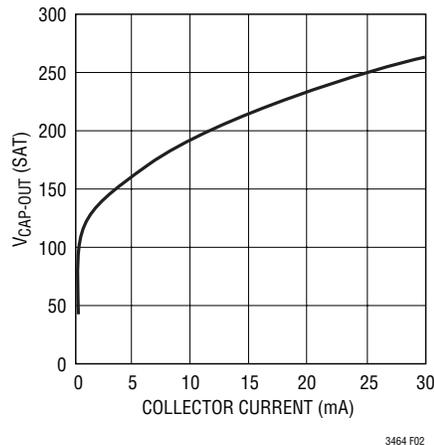
Figure 5: Output Disconnect Voltage Drop ( $V_{DROPP}$ ) vs Current
