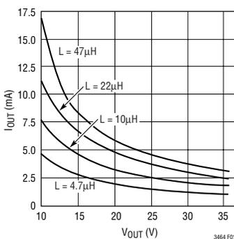
**Figure 1. Maximum Output Current**
