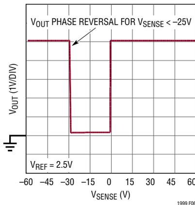
Figure 7. A Plot of the LT1999's Output Voltage vs  $V_{SENSE}$  ( $V_{SENSE} = V_{+IN} - V_{-IN}$ ). In Applications Where the Sense Voltage Is Driven in Excess of  $-25V$ , the Output of the LT1999 Will Undergo Phase Reversal
