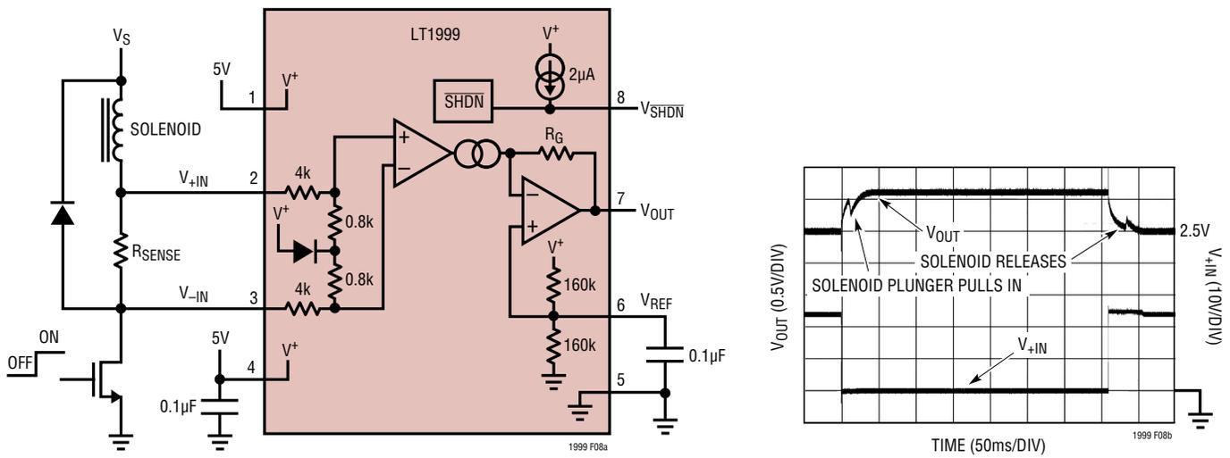
**Figure 9. Solenoid Current Monitor for Non-Grounded Solenoids. This Circuit Performs the Same Function as Figure 7 Except One End of the Solenoid Is Tied to V<sub>S</sub>. The Common Mode Voltage of Inputs of the LT1999 Switch Between Ground and One Diode Drop Above V<sub>S</sub>**
