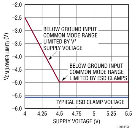
Figure 3. Lower Input Common Mode vs Supply Voltage
