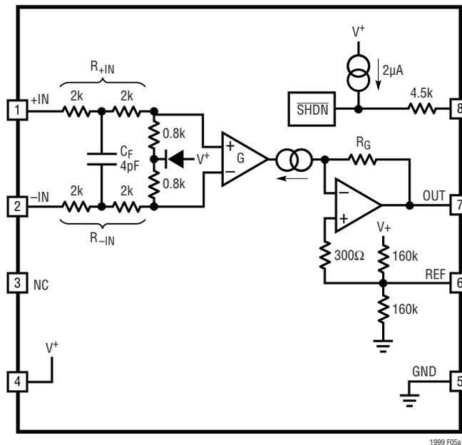
Figure 5. Simplified Block Diagram of the LT1999-XXF
