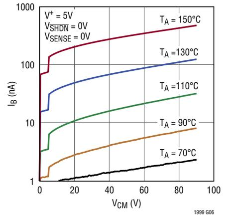
**Input Bias Current vs Input Common Mode**
