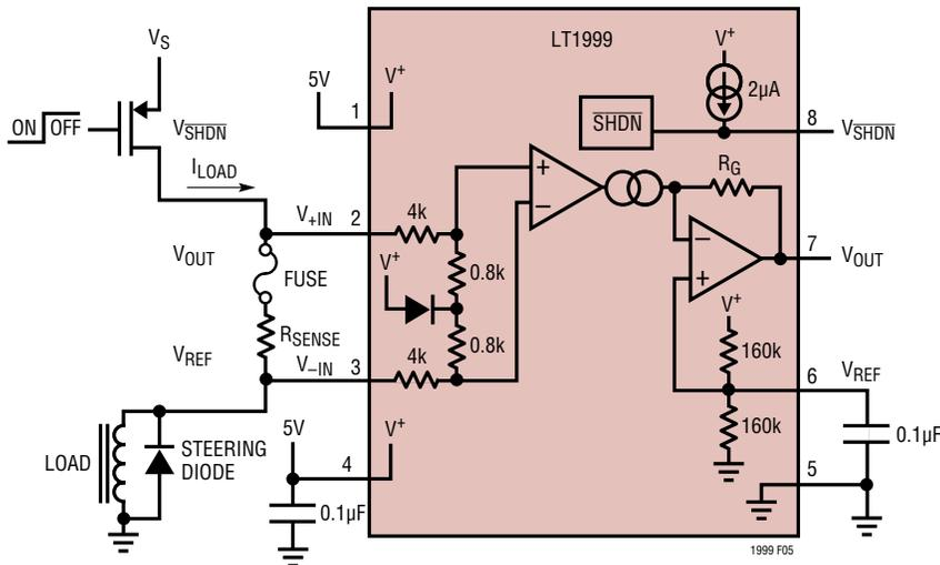
Figure 6. Using the LT1999 to Monitor a Fuse
