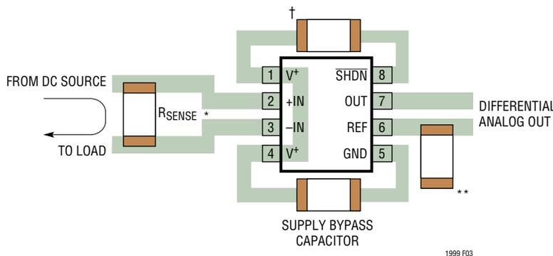
\* KEEP LOOP AREA COMPRISING  $R_{\text{SENSE}}$ , +IN AND -IN PINS AS SMALL AS POSSIBLE.
