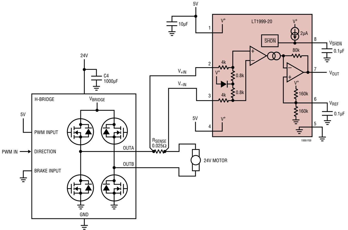
**Figure 10. Armature Current Monitor for DC Motor Applications**
