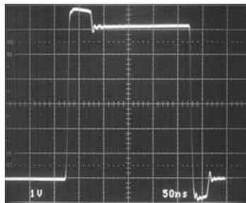
Large-Signal Transient,  $A_V = 1, C_L = 1000\text{pF}$
