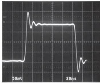
Small-Signal Transient,  $A_V = 1, C_L = 1000\text{pF}$
