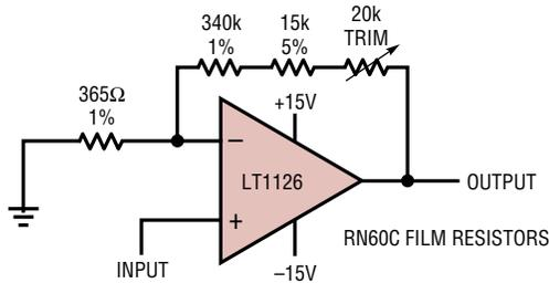
THE HIGH GAIN AND WIDE BANDWIDTH OF THE LT1126/LT1127 IS USEFUL IN LOW FREQUENCY HIGH CLOSED LOOP GAIN AMPLIFIER APPLICATIONS. A TYPICAL PRECISION OP AMP MAY HAVE AN OPEN LOOP GAIN OF ONE MILLION WITH 500kHz BANDWIDTH. AS THE GAIN ERROR PLOT SHOWS, THIS DEVICE IS CAPABLE OF 0.1% AMPLIFYING ACCURACY UP TO 0.3Hz ONLY. EVEN INSTRUMENTATION RANGE SIGNALS CAN VARY AT A FASTER RATE. THE LT1126/LT1127 "GAIN PRECISION — BANDWIDTH PRODUCT" IS 330 TIMES HIGHER, AS SHOWN.
