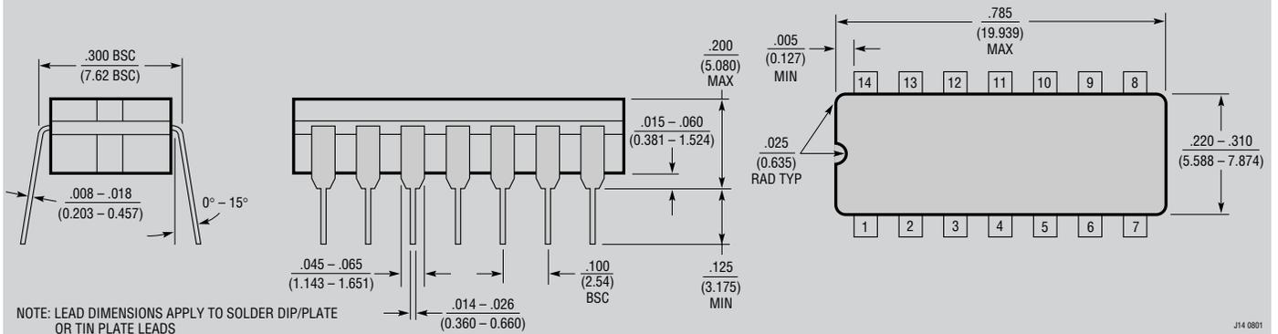
NOTE: LEAD DIMENSIONS APPLY TO SOLDER DIP/PLATE OR TIN PLATE LEADS
