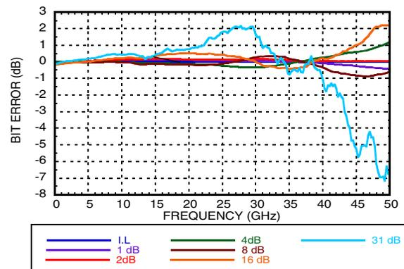
**1.0 dB LSB GaAs MMIC 5-BIT DIGITAL ATTENUATOR, 0.1 - 40 GHz**
