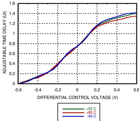
**Time Delay vs. Control Voltage**
