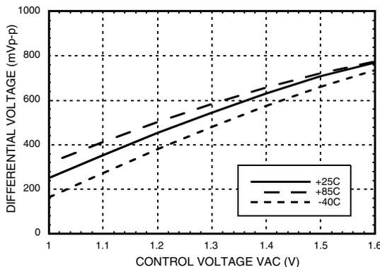
**Differential Output vs. Vin & Temperature @ 16 GHz [1][2]**
