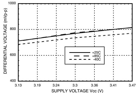
**Differential Output vs. Control Voltage [2]**
