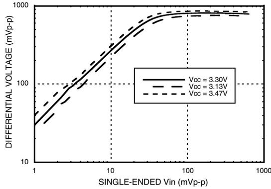
**Differential Output vs. Vininput & Frequency [1] [2]**
