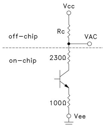
The value of the resistor can be chosen using the following equation as a function of VAC. VAC DC voltage value can be chosen by using the plot given above.
