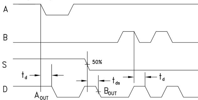
$t_d$  = propagation delay, A to D
