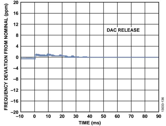
Figure 40. DAC Assisted Release
