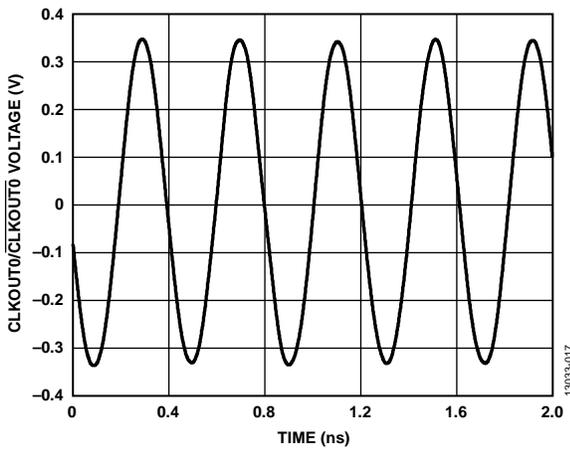
Figure 16. Differential CLKOUT0/CLKOUT0 at 2457 MHz, LVPECL
