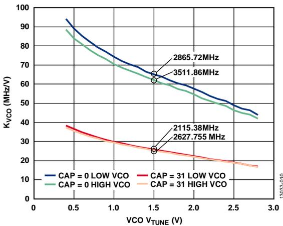
Figure 11. VCO Gain ( $K_{VCO}$ ) vs. VCO  $V_{TUNE}$
