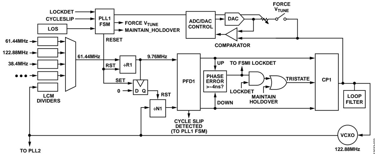
Figure 36. PLL1 Architecture with a Typical Frequency Configuration
