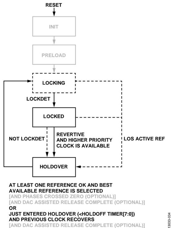
Figure 37. PLL1 FSM Simplified State Diagram—
