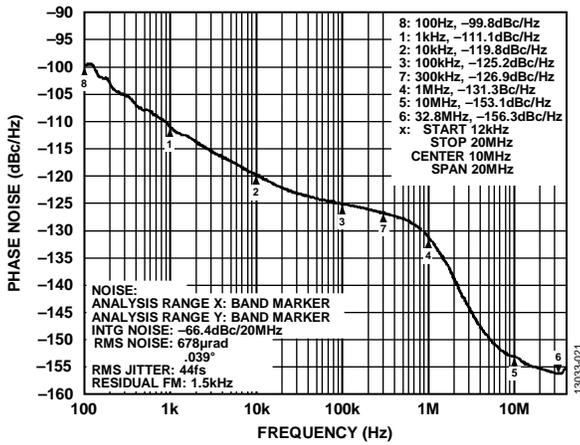
Figure 10. Phase Noise,  $\overline{CLKOUTx}/\overline{CLKOUTx} = 2457.6$  MHz, Optimized for Best Integrated Jitter (12 kHz to 20 MHz)
