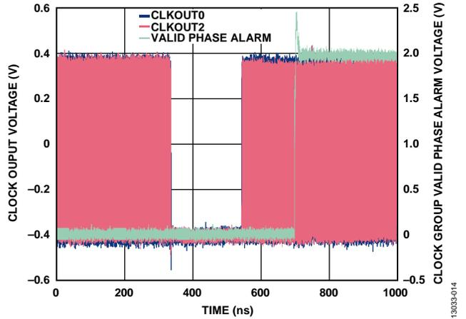
Figure 24. Output Channel Synchronization Before and After Rephase
