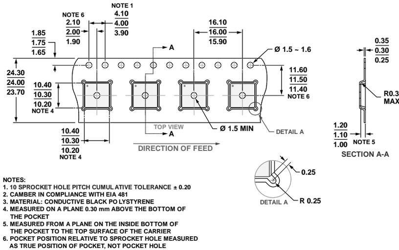
Figure 55. LFCSP Tape and Reel Outline Dimensions
