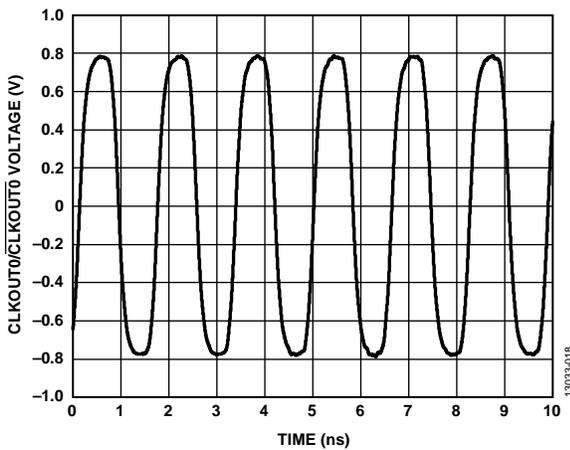
Figure 17. Differential CLKOUT0/CLKOUT0 Voltage at 614.4 MHz, LVPECL
