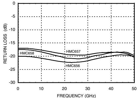
[2] Data taken with die mounted to plate and RF probed through two 3 x 0.5 mil ribbon bonds.
