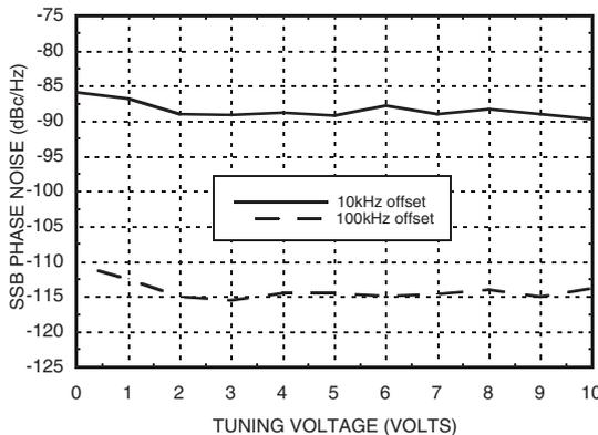
**Typical SSB Phase Noise @  $V_{tune} = +5V$**
