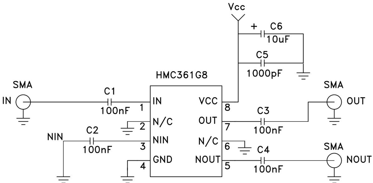
Capacitors C1, C2, C3, and C4 are broadband multilayer capacitors, American Technical Ceramics part number ATC530L. The 100 nF capacitance value is per ATC datasheet.
