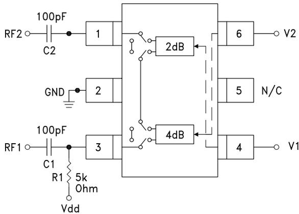
DC blocking capacitors C1 & C2 are required on RF1 & RF2. Choose C1 = C2 = 100 ~ 300 pF to allow lowest customer specific frequency to pass with minimal loss. R1 = 5K Ohm is required to supply voltage to the circuit through either PIN 3 or PIN 1.
