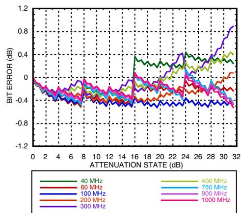
**Bit Error vs. Frequency<sup>[1][2]</sup>**
