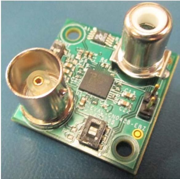
Figure 5. EVAL-CN0428-EBZ Water Sensor Boards
