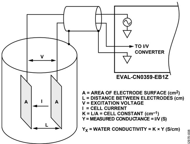
Figure 8. Interface Between Conductivity Cell and EVAL-CN0359-EB1Z
