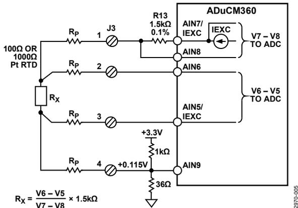
Figure 5. Configuration for 4 Wire RTD Connection
