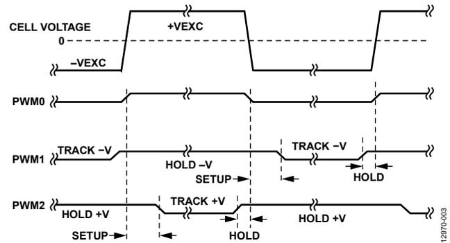
Figure 3. Cell Voltage and Track-and-Hold Timing Signals
