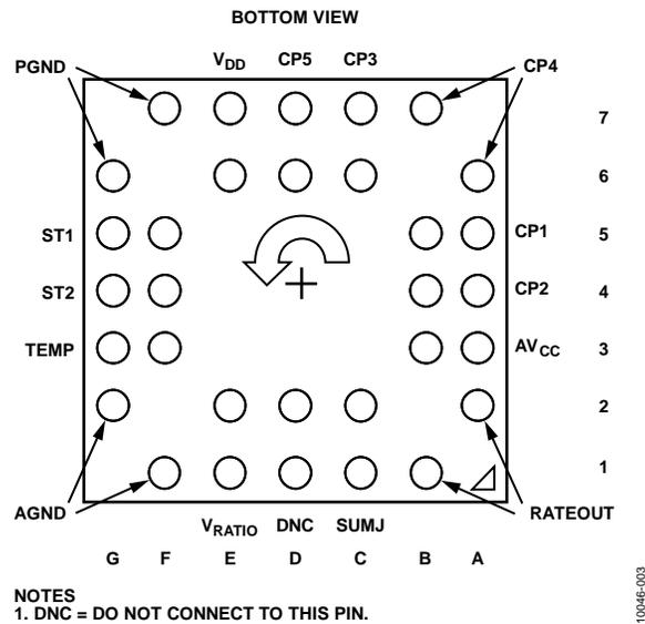
Figure 3. Pin Configuration
