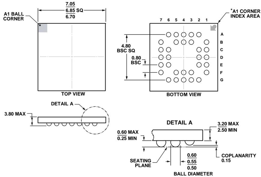
\*BALL A1 IDENTIFIER IS GOLD PLATED AND CONNECTED TO THE D/A PAD INTERNALLY VIA HOLES.
