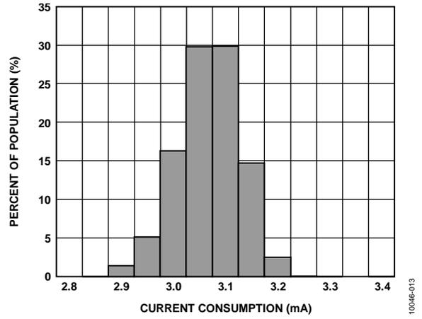
Figure 18. Current Consumption at 25°C (V<sub>RATIO</sub> = 5 V)
