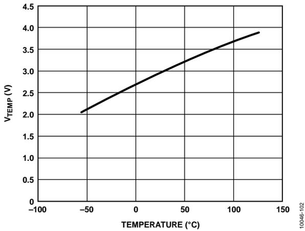
Figure 17. V<sub>TEMP</sub> Output vs. Temperature
