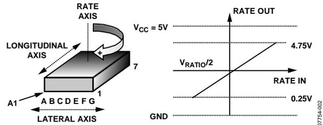
Figure 2. RATEOUT Signal Increases with Clockwise Rotation
