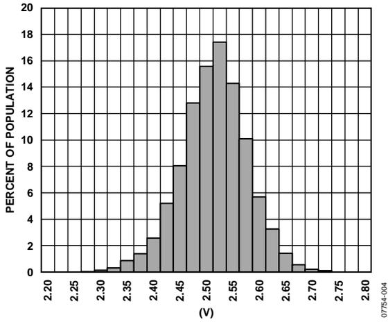
Figure 4. Null Output at 25°C ( $V_{RATIO} = 5 V$ )
