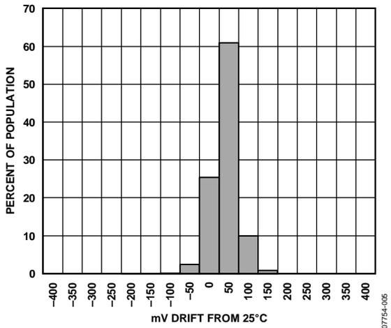
Figure 5. Null Drift over Temperature ( $V_{RATIO} = 5 V$ )
