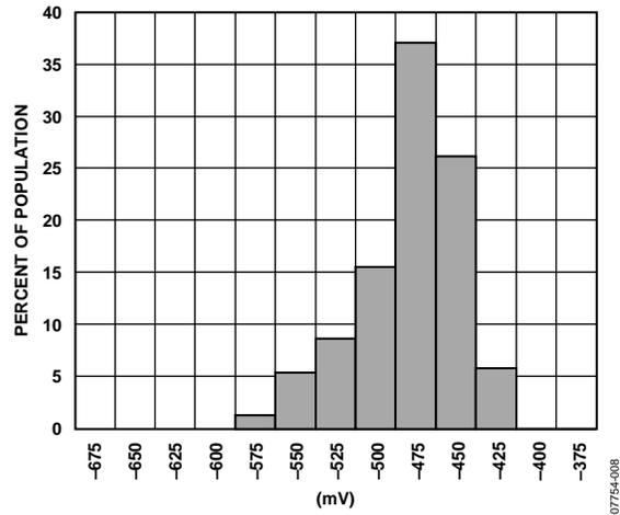
Figure 8. ST1 Output Change at 25°C ( $V_{RATIO} = 5 V$ )
