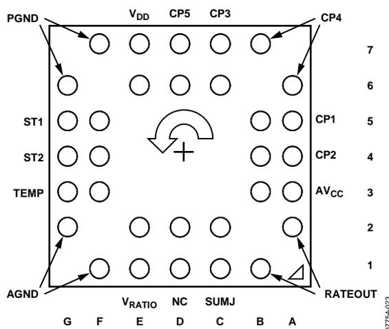
Figure 3. Pin Configuration
