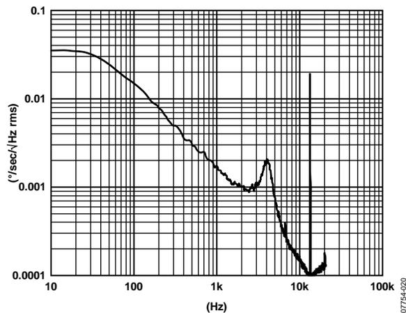
Figure 21. Typical Noise Spectral Density (Bandwidth = 40 Hz)
