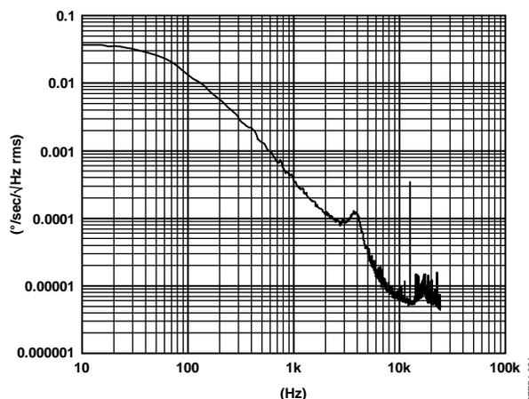
Figure 22. Noise Spectral Density with Additional 250 Hz Filter
