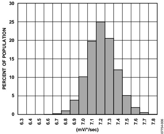
Figure 6. Sensitivity at 25°C ( $V_{RATIO} = 5 V$ )
