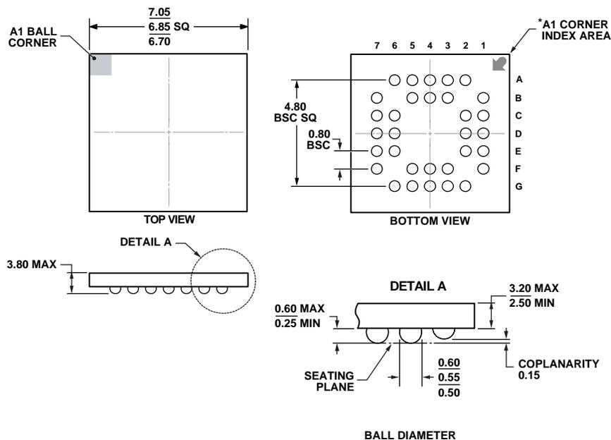
\*BALL A1 IDENTIFIER IS GOLD PLATED AND CONNECTED TO THE D/A PAD INTERNALLY VIA HOLES.
