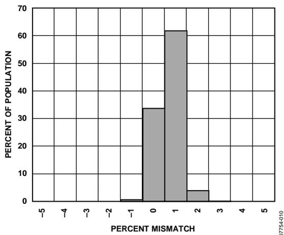
Figure 10. Self-Test Mismatch at 25°C ( $V_{RATIO} = 5 V$ )
